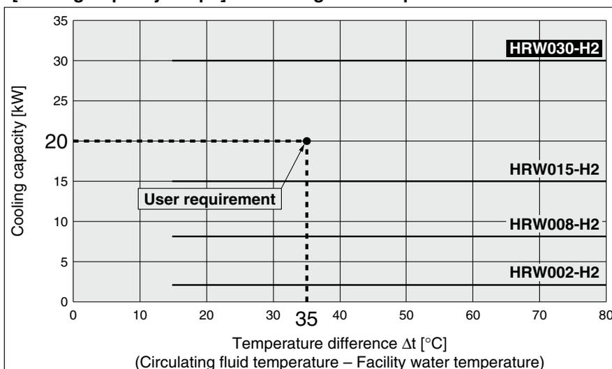
The point plotted in the graph is the requirement from the user. Select the thermo-chiller models exceeding this point. In this case, select the **HRW030-H2**.
