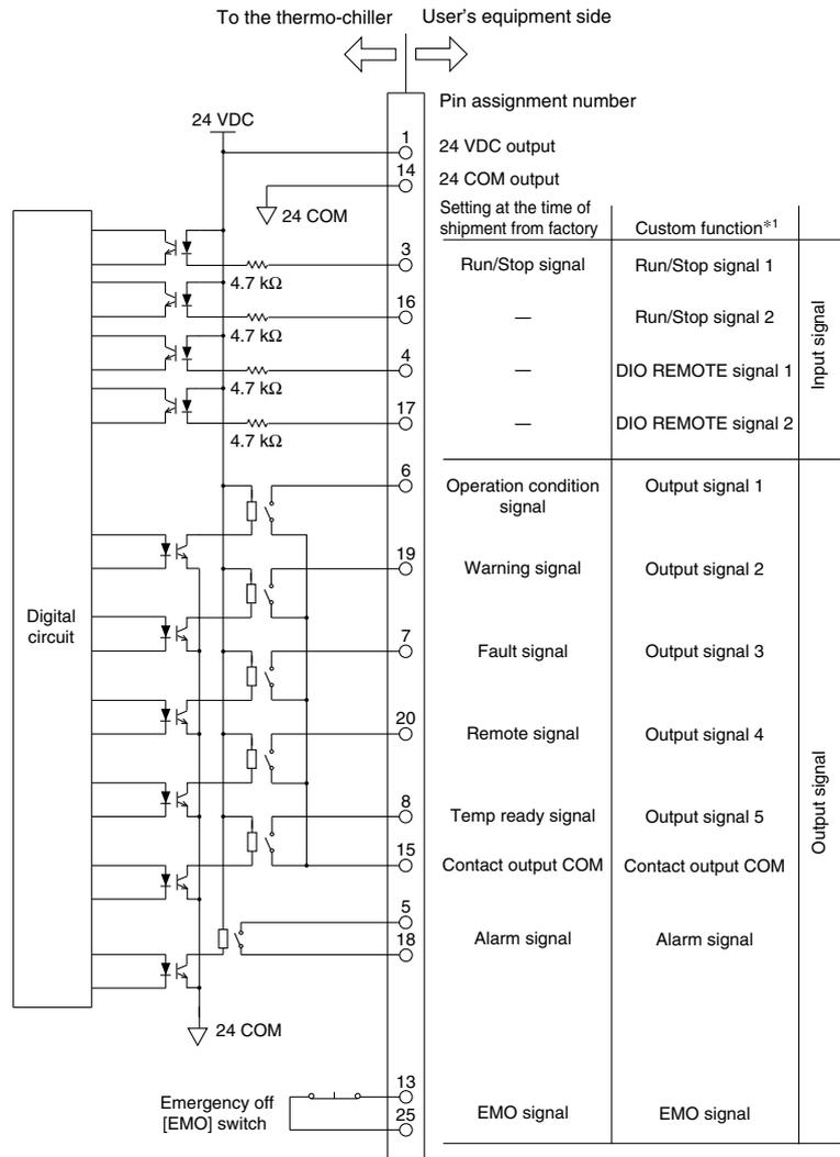
\*1 The custom function is equipped for contact input/output. Using the custom function enables the user to set the signal type for contact input/output or pin assignment numbers. For details, please refer to the "Communication Specifications" information.
