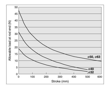
• A case where the center of gravity of the load rests 50 mm from the rod end.
