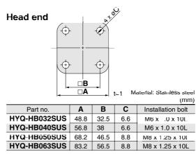
Note) One mounting bracket is attached with four mounting bolts
