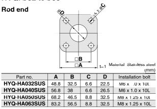
Note) One mounting bracket is attached with four mounting bolts
