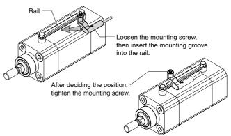
Tighten the screw within the following torque range when the auto switch mounting rail is installed during maintenance.
