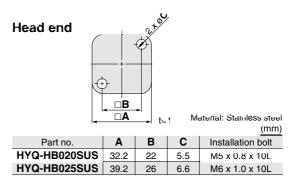
Note) One mounting bracket is attached with two mounting bolts.
