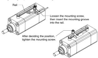
Tighten the screw within the following torque range when the auto switch mounting rail is installed during maintenance.
