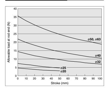
• A case where the center of gravity of the load rests 50 mm from the rod end.
