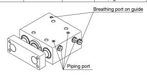
3. Use the piping tube installed in the breathing port for guide is more than ø4 in bore size and within 3 m in length, otherwize the cylinder piston speed might decrease.
