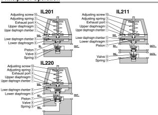
The signal air pressure enters the upper diaphragm chamber ① to generate a force. When this force is larger than the force generated by compressing the adjusting spring ③, the upper diaphragm ② is pushed up, the exhaust port ④ is closed, and the signal air pressure enters the lower diaphragm chamber ③ and acts the lower diaphragm ⑥. This pushes down the piston ⑦ to open the valve.
