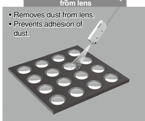
Neutralizing static electricity from lens
