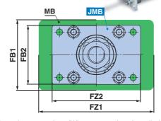
Width: Max. 20 % reduction, Height: 16 % reduction Dimension comparison (When mounted on the cylinder)
