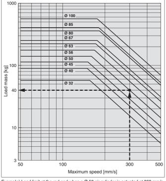
Example) Load limit at the rod end when a  $\emptyset$  50 air cylinder is actuated at 300 mm/s Extend upward from 300 mm/s on the horizontal axis of the graph to the intersection point with the line for a 50 mm bore size, and then extend leftward from this point to find the load of 40 kg.
