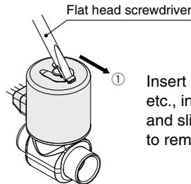
Insert a flat head screwdriver, etc., into the groove in the clip and slide it in the direction of ① to remove it.
