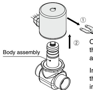
Once the clip has been removed, the coil can be removed from above (in the direction of ②).
