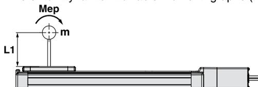
Selection example) Select the **LEJS63V7B-300** from the graph on the right side. Confirm that the external force is 20 [N] or less. (The external force is the resistance due to cable duct, flexible trunking or air tubing.)
