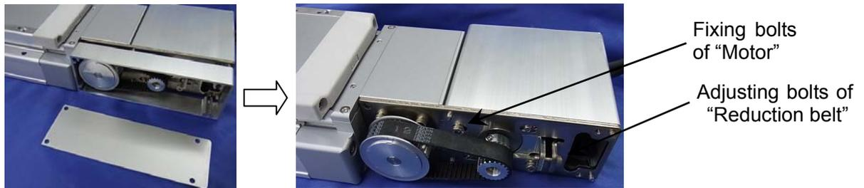
Table 6-2. Fixing bolts of “Motor”
