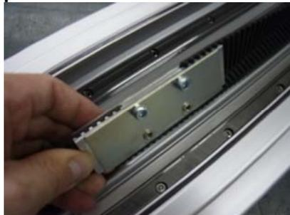
7-8. Fix the "Belt holder" to the "Table", then attach the "Table cap".
