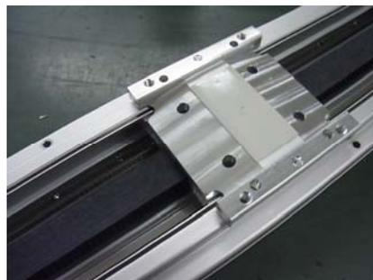
7-9. After adjusting tension of the "Drive belt", plug the "Dust seal band" of the end side.
