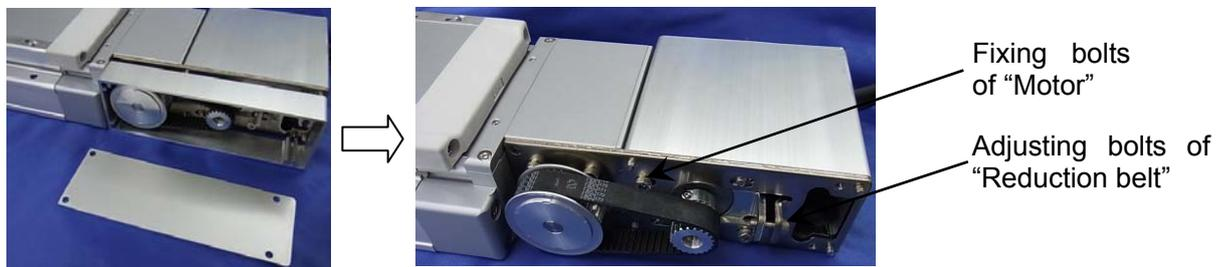
Table 8-2. Fixing bolts of “Motor”
