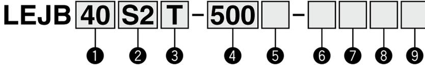
The LECSB-S, LECS-C-S, and LECS-S-S electric actuator drivers are to be discontinued. The LECSB-T, LECS-C-T, and LECS-S-T drivers are available as substitutes. In the product number, select T6 instead of S6, or T7 instead of S7 for the ② Motor type, and select B2 instead of B1, C2 instead of C1, or S2 instead of S1 for the ③ Driver type.
