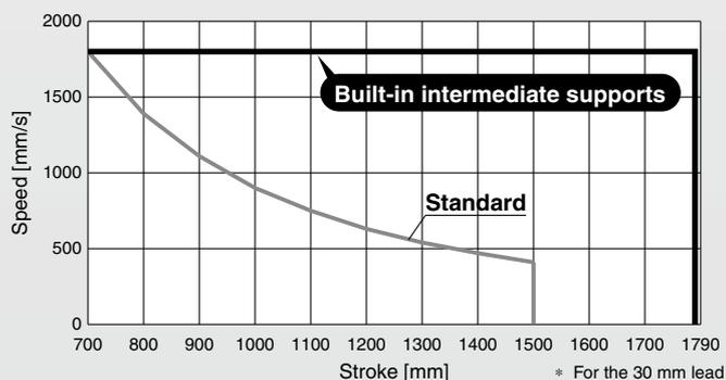
The use of intermediate supports results in reduced deflection of the ball screw when a long stroke is used.
