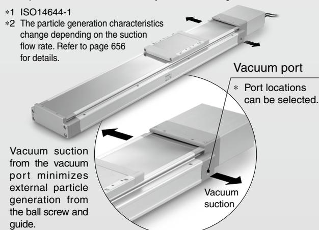
Vacuum suction from the vacuum port minimizes external particle generation from the ball screw and guide.
