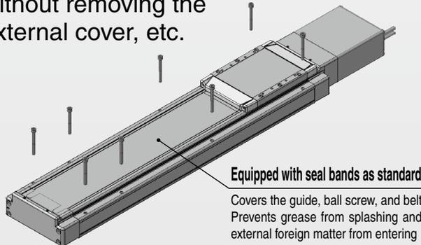
Equipped with seal bands as standard
