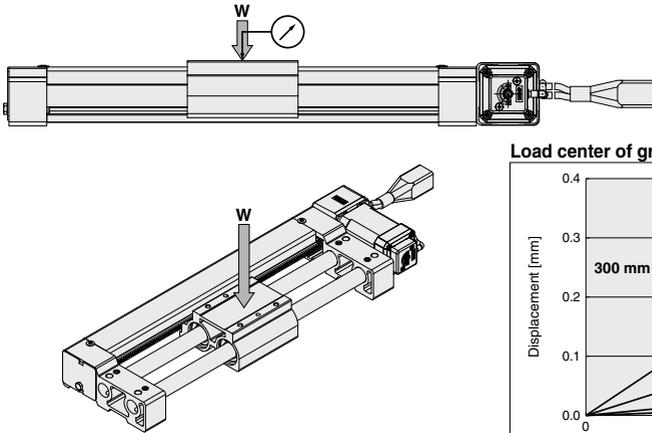
Load center of gravity located at the center of the table
