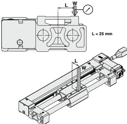
Load center of gravity located at a position offset when L = 25 mm
