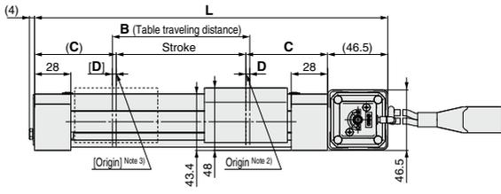
Note 1) Distance within which the table can move when it returns to origin. Make sure a workpiece mounted on the table does not interfere with the workpieces and facilities around the table.
