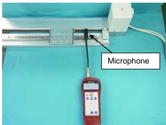
Recommended position of the belt tension meter
