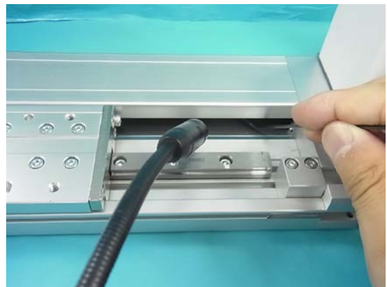
Tap the belt with a thin rod such as a hexagon wrench at the specified position for tensile measurement. Do not use a rod which has a sharp edge, as it may damage the belt.
