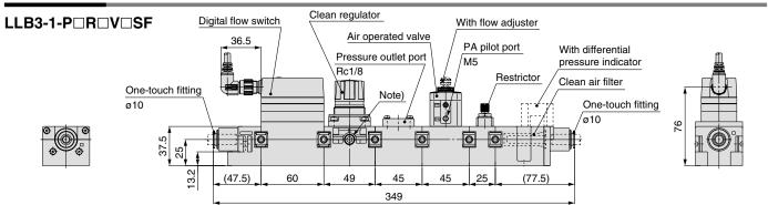
Note) This port is unavailable. If a pressure gauge, etc. is screwed in, the port may be damaged.
