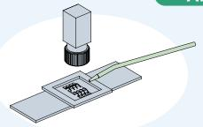
N<sub>2</sub> blow to prevent lead frame oxidation, N<sub>2</sub> blow to prevent detection camera blur
