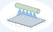
Prevents traces of water droplets. Air-knife
