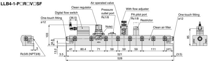
Note) This port is unavailable. If a pressure gauge, etc. is screwed in, the port may be damaged.
