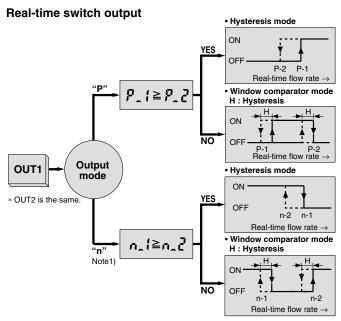
Note 1) The output mode is set to the inverted output when shipped from the factory.
