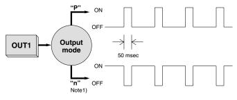
Note 1) The output mode is set to the inverted output when shipped from the factory. Note 2) Refer to the specifications of display unit for the flow rate value per pulse.
