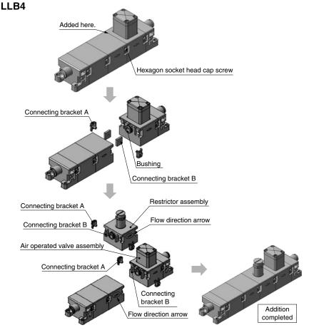
Example: Addition of the restrictor assembly (LVB4-4)
