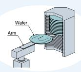
Suction/release air for wafer-transfer robot
