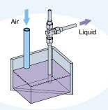
Compressed air for lifting clean liquid
