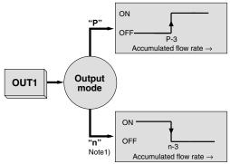
Note 1) The output mode is set to the inverted output when shipped from the factory.
