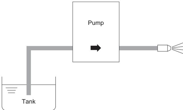
2. Make sure to remove any air bubbles in the piping and pump chamber before use.
