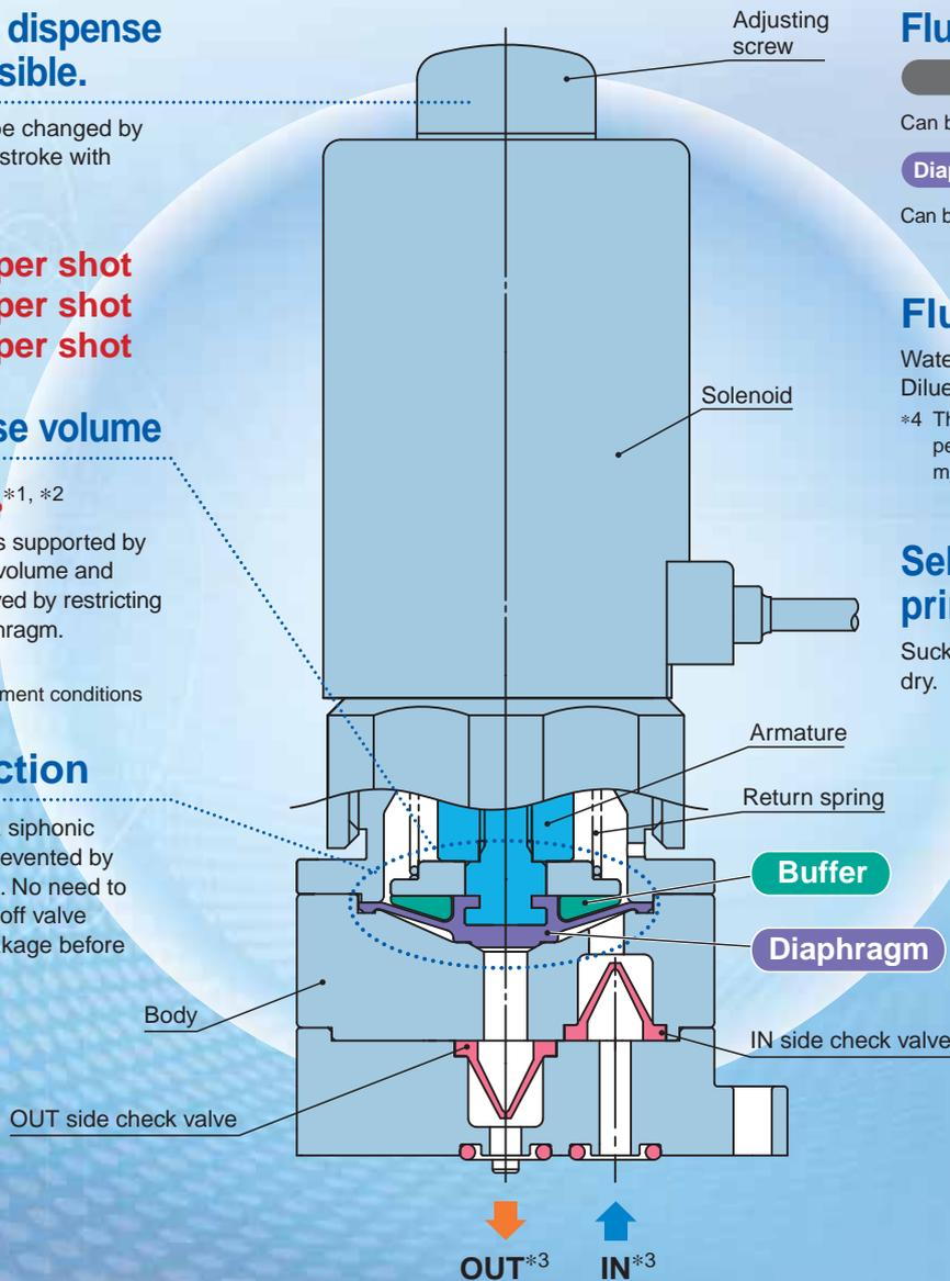
\*3 Do not apply positive or vacuum pressure to IN or OUT port.
