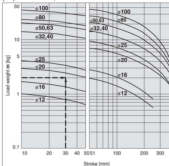
· When the maximum speed exceeds 200 mm/s, the allowable load weight is determined by multiplying the value shown in the graph at 400 mm/s by the coefficient listed in the table below.
