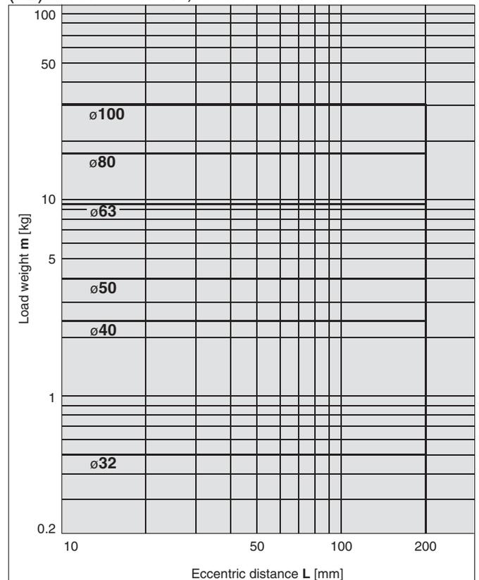
· Use the "Guide Cylinder Selection Software", when the eccentric distance is 200 mm or more.
