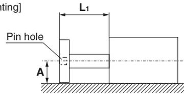
$$A = \text{[Catalogue dimension]} \pm^* (0.1 + L_1 \times 0.0008) \text{ [mm]}$$
