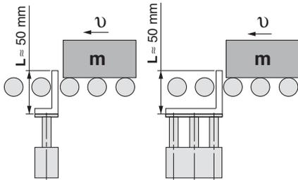
\* When selecting a model with a longer L dimension, be sure to choose a bore size which is sufficiently large.
