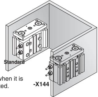
This makes it easy to remove and rotate piping when it is mounted on a wall where mounting space is limited.
