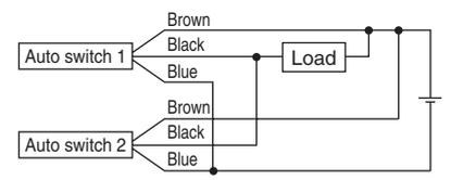
The indicator lights will light up when both of the auto switches are in the ON state.
