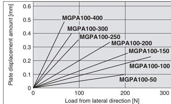
Note 1) The guide rod and self-weight for the plate are not included in the above displacement values.
