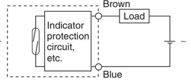
(Power supply for switch and load are separate.)
