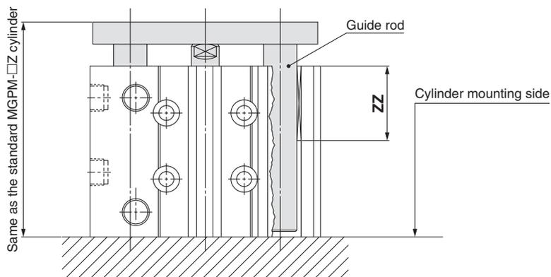
Note) The total length (ZZ) of the guide rod bushing is shorter than the standard type.
