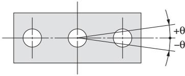
Non-rotating accuracy  $\theta$  when retracted and when no load is applied should be not more than the values shown in the table.
