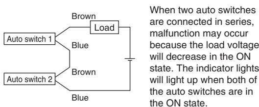
When two auto switches are connected in series, malfunction may occur because the load voltage will decrease in the ON state. The indicator lights will light up when both of the auto switches are in the ON state.
