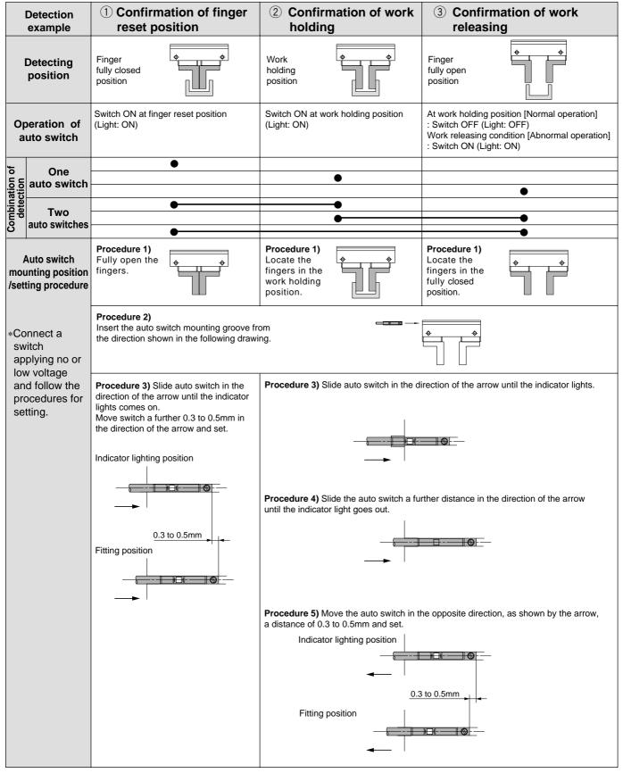
Note) •It is recommended that work be held at the center of the finger stroke.
