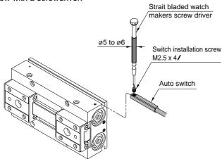
Note) Use a screwdriver with a grip diameter of 5 to 6 mm to tighten the auto switch mounting screw. The tightening torque should be about 0.05 to 0.1N·m. When you begin to feel that the screw is being tightened, turn it further by 90°.
