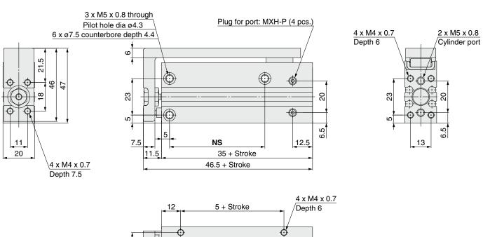
Note 1) Refer to "Specific Product Precautions" for mounting of the Compact Slide and a workpiece. Note 2) When changing the port location, please order a new port plug: MXH-P (2 pcs.)
