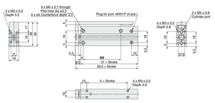
Note 1) Refer to "Specific Product Precautions" for mounting of the Compact Slide and a workpiece. Note 2) When changing the port location, please order a new port plug: MXH-P (2 pcs.)
