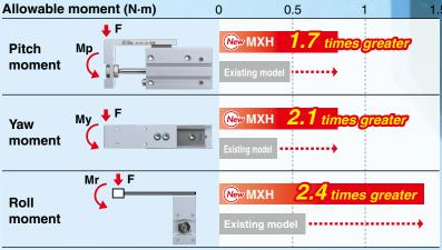
\* Allowable moment caused by static load
