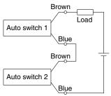
When two auto switches are connected in series, a load may malfunction because the load voltage will decline when in the ON state. The indicator lights will light up when both of the auto switches are in the ON state. Auto switches with load voltage less than 20V cannot be used.
