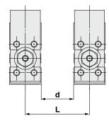
Dimensions of a shielding plate (MU-S025) that is sold separately are indicated as reference.
