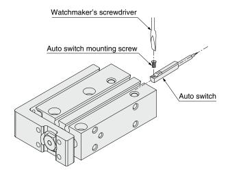
When tightening the auto switch mounting screw, use a watchmaker's screwdriver with a handle 5 to 6 mm in diameter.
