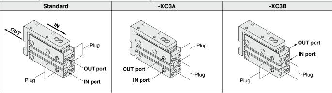
3 Intermediate stroke (Spacer type)
