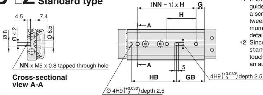
\*1 If long bolts are used, they may touch the guide block and cause a malfunction, etc. Use a screw which has an intermediate length between the maximum screw-in depth and minimum screw-in depth. Refer to page 196 for details.
