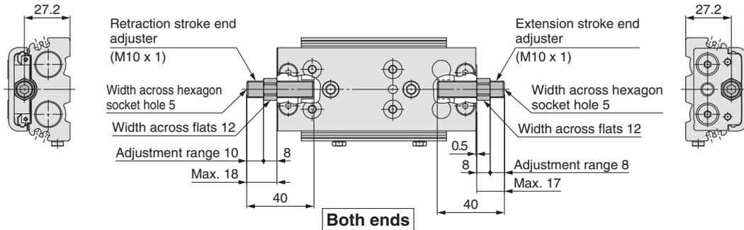
Rubber stopper **ZD**: Both ends, **ZE**: Extension stroke end, **ZF**: Retraction stroke end, **ZP**: Retraction stroke end (Shorter total length type)
