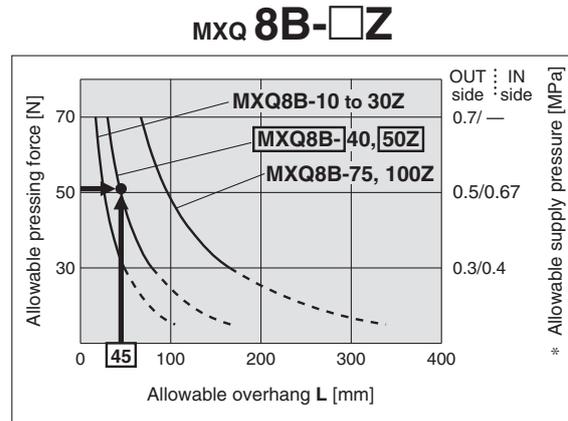
\* The allowable supply pressure on the OUT side and IN side is the theoretical output of the cylinder when pressing force is required.
