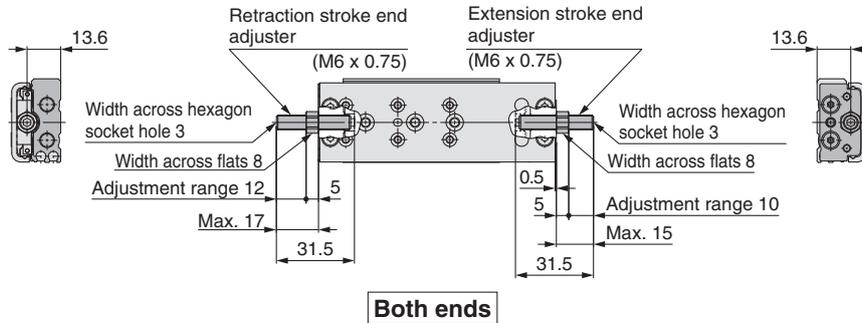
Shock absorber/RJ **ZG**: Both ends, **ZH**: Extension stroke end, **ZJ**: Retraction stroke end, **ZQ**: Retraction stroke end (Shorter total length type)
