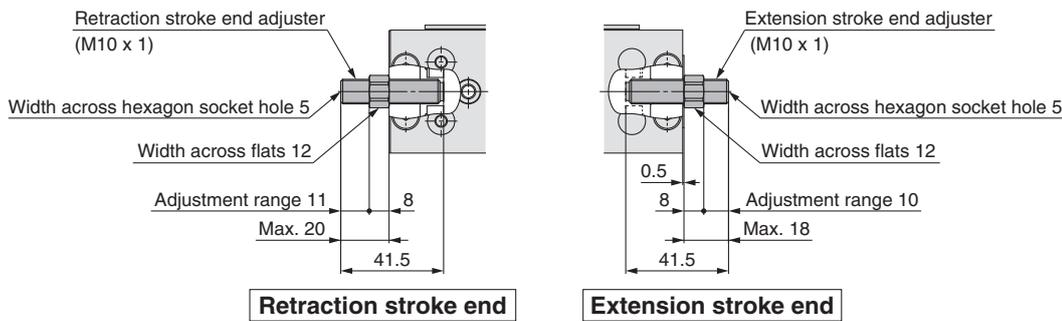
Shock absorber/RJ **ZG**: Both ends, **ZH**: Extension stroke end, **ZJ**: Retraction stroke end, **ZQ**: Retraction stroke end (Shorter total length type)
