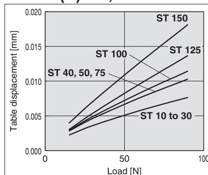
**Table displacement due to roll moment load**
