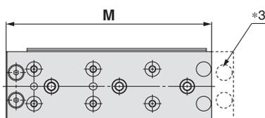
\*3 As the total length has been reduced by removing the extension stroke end adjuster mounting holes, an extension stroke end adjuster cannot be mounted afterward. (Retraction stroke end adjusters can be mounted afterward.)
