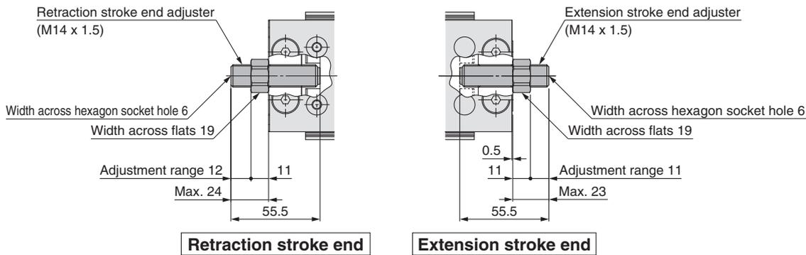
Shock absorber/RJ **ZG**: Both ends, **ZH**: Extension stroke end, **ZJ**: Retraction stroke end, **ZQ**: Retraction stroke end (Shorter total length type)
