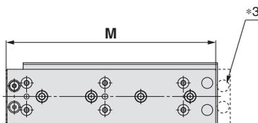
\*3 As the total length has been reduced by removing the extension stroke end adjuster mounting holes, an extension stroke end adjuster cannot be mounted afterward. (Retraction stroke end adjusters can be mounted afterward.)
