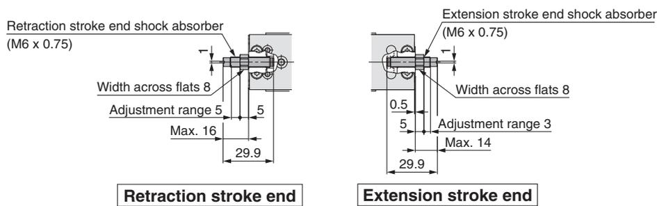
Metal stopper **ZK**: Both ends, **ZL**: Extension stroke end, **ZM**: Retraction stroke end, **ZT**: Retraction stroke end (Shorter total length type)
