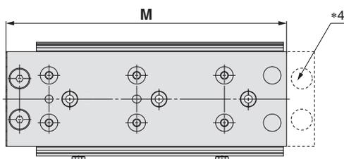
\*4 As the total length has been reduced by removing the extension stroke end adjuster mounting holes, an extension stroke end adjuster cannot be mounted afterward. (Retraction stroke end adjusters can be mounted afterward.)
