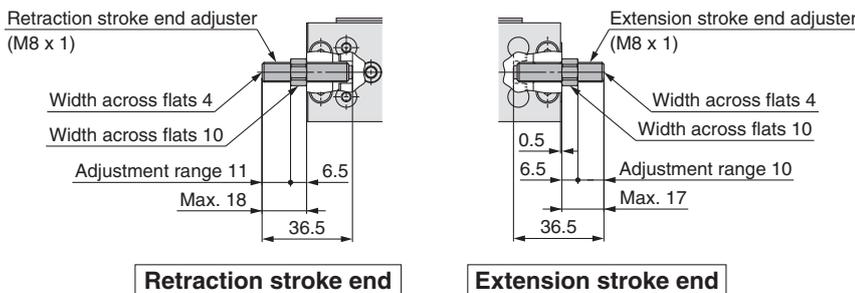
Shock absorber/RJ **ZG**: Both ends, **ZH**: Extension stroke end, **ZJ**: Retraction stroke end, **ZQ**: Retraction stroke end (Shorter total length type)
