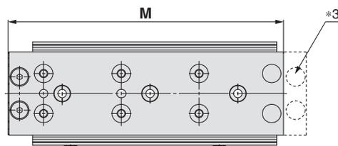
\*3 As the total length has been reduced by removing the extension stroke end adjuster mounting holes, an extension stroke end adjuster cannot be mounted afterward. (Retraction stroke end adjusters can be mounted afterward.)
