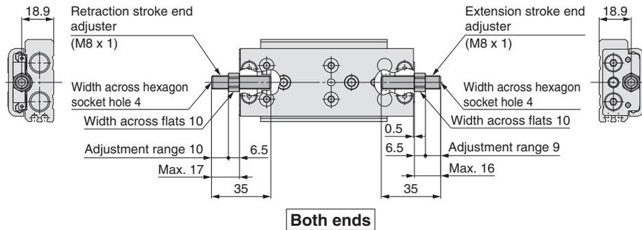
Rubber stopper **ZD**: Both ends, **ZE**: Extension stroke end, **ZF**: Retraction stroke end, **ZP**: Retraction stroke end (Shorter total length type)
