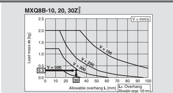
This product can be used with the overhang required (L1, L2, L3 of No.3) if it is within the allowable overhang range (L1max, L2max, L3max of No.4).
