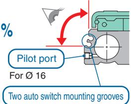
■ A piping port and auto switch mounting groove are provided on both sides.
