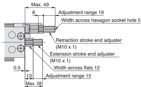
Shock absorber/RJ **ZG**: Both ends,
