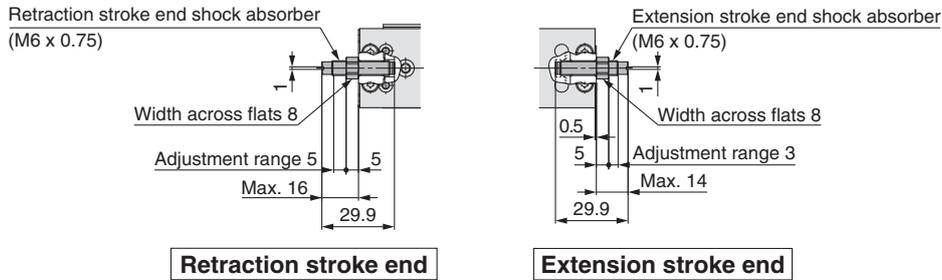
Metal stopper **ZK**: Both ends, **ZL**: Extension stroke end, **ZM**: Retraction stroke end, **ZT**: Retraction stroke end (Shorter total length type)
