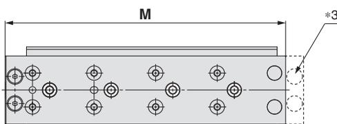
\*3 As the total length has been reduced by removing the extension stroke end adjuster mounting holes, an extension stroke end adjuster cannot be mounted afterward. (Retraction stroke end adjusters can be mounted afterward.)
