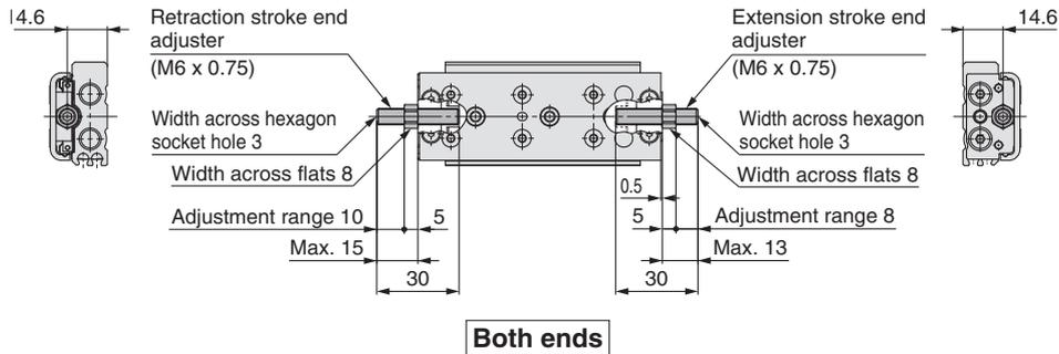
Rubber stopper **ZD**: Both ends, **ZE**: Extension stroke end, **ZF**: Retraction stroke end, **ZP**: Retraction stroke end (Shorter total length type)
