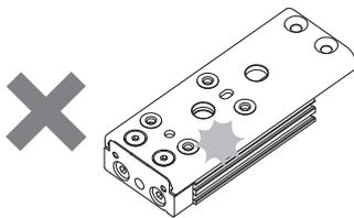
3. Do not apply excessive impact or loads when a workpiece is mounted.
