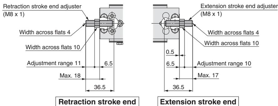
Shock absorber/RJ **ZG**: Both ends, **ZH**: Extension stroke end, **ZJ**: Retraction stroke end, **ZQ**: Retraction stroke end (Shorter total length type)
