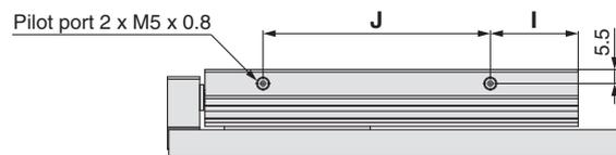
\*1 If long bolts are used, they may touch the guide block and cause a malfunction, etc. Use a screw which has an intermediate length between the maximum screw-in depth and minimum screw-in depth. Refer to page 196 for details.
