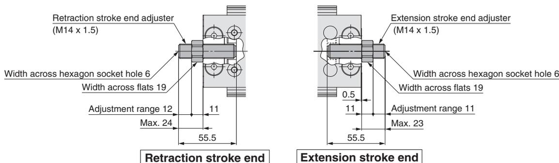
Shock absorber/RJ **ZG**: Both ends, **ZH**: Extension stroke end, **ZJ**: Retraction stroke end, **ZQ**: Retraction stroke end (Shorter total length type)
