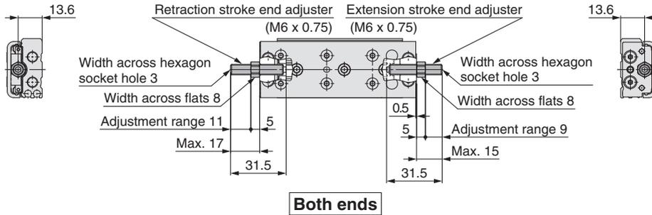
Shock absorber/RJ **ZG**: Both ends, **ZH**: Extension stroke end, **ZJ**: Retraction stroke end, **ZQ**: Retraction stroke end (Shorter total length type)
