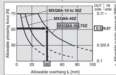
\* The allowable supply pressure on the OUT side and IN side is the theoretical output of the cylinder when pressing force is required.
