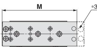
\*3 As the total length has been reduced by removing the extension stroke end adjuster mounting holes, an extension stroke end adjuster cannot be mounted afterward. (Retraction stroke end adjusters can be mounted afterward.)
