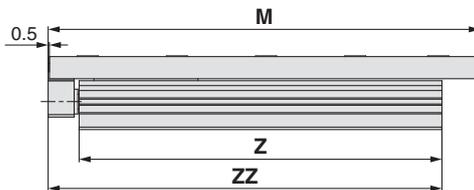
\*1 If long bolts are used, they may touch the guide block and cause a malfunction, etc. Use a screw which has an intermediate length between the maximum screw-in depth and minimum screw-in depth. Refer to page 196 for details.
