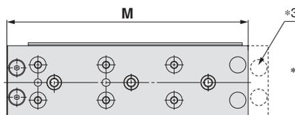
\*3 As the total length has been reduced by removing the extension stroke end adjuster mounting holes, an extension stroke end adjuster cannot be mounted afterward. (Retraction stroke end adjusters can be mounted afterward.)
