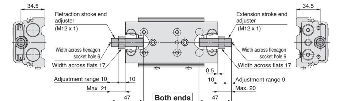
Rubber stopper **ZD**: Both ends, **ZE**: Extension stroke end, **ZF**: Retraction stroke end, **ZP**: Retraction stroke end (Shorter total length type)
