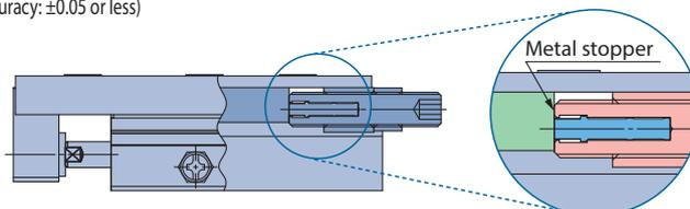
It is possible to combine an extension stroke end adjuster and a retraction stroke end adjuster.
