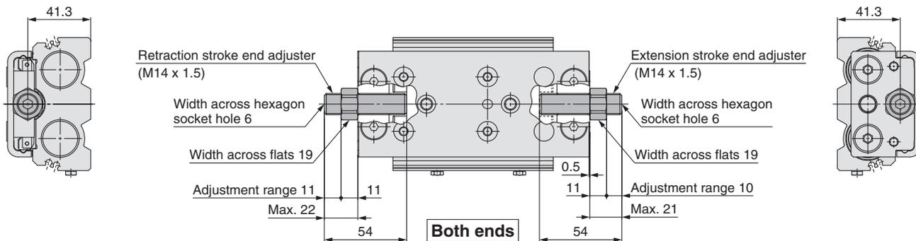
Rubber stopper **ZD**: Both ends, **ZE**: Extension stroke end, **ZF**: Retraction stroke end, **ZP**: Retraction stroke end (Shorter total length type)
