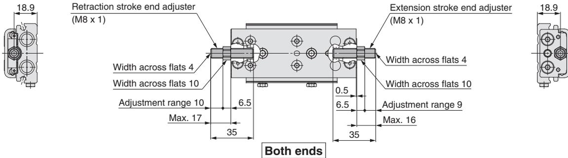
Rubber stopper **ZD**: Both ends, **ZE**: Extension stroke end, **ZF**: Retraction stroke end, **ZP**: Retraction stroke end (Shorter total length type)
