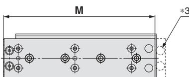
\*3 As the total length has been reduced by removing the extension stroke end adjuster mounting holes, an extension stroke end adjuster cannot be mounted afterward. (Retraction stroke end adjusters can be mounted afterward.)
