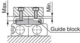
**⚠ Caution** In order to prevent the workpiece fixing bolt from hitting the table, use a bolt of a length at least 0.5 mm shorter than the maximum screw-in depth. If long bolts are used, they may touch the guide block and cause a malfunction, etc.
