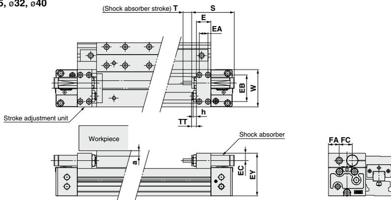
\* Since the EY dimension of H unit is greater than the table top height (H dimension), when a work piece exceeding the full length (L dimension) of the slide table is mounted, allow a clearance of size "a" or larger at the work piece side.
