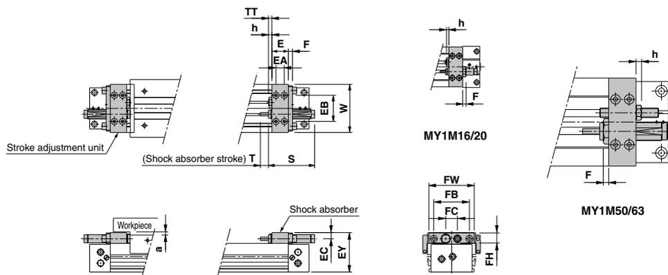
\* Since dimension EY of the H type unit is greater than the table top height (dimension H), when mounting a workpiece that exceeds the overall length (dimension L) of the slide table, allow a clearance of dimension "a" or larger on the workpiece side.
