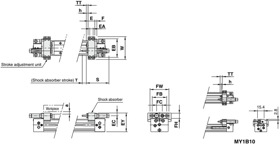
\* Since the dimension EY of H unit is greater than the table top height (dimension H), when a workpiece is loaded that is larger than the full length (dimension L) of the slide table allow a clearance of size "a" or larger at the workpiece side. (mm)
