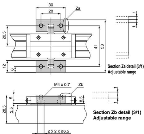
Note) A set of brackets with floating mechanism consists of a left bracket and a right bracket.
