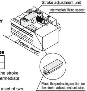
\* When ordering the intermediate fixing spacer for the stroke adjustment unit, the intermediate fixing spacer is shipped together.
