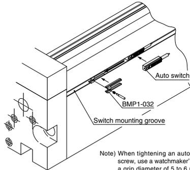
Note) When tightening an auto switch mounting screw, use a watchmaker's screwdriver with a grip diameter of 5 to 6 mm. Also, tighten with a torque of about 0.05 to 0.1 N·m. As a guide, it should be turned about 90° past the point at which tightening can be felt.
