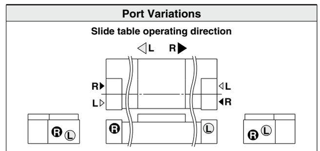
**Standard Type/Centralized Piping Type  $\phi 16, \phi 20$**
