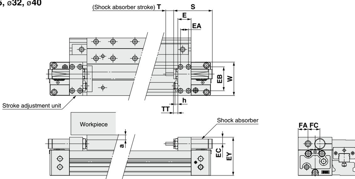
\* Since the EY dimension of H unit is longer than the table top height (H dimension), when mounting a workpiece that exceeds the overall length (L dimension) of the slide table, allow a clearance of dimension "a" or longer on the workpiece side.
