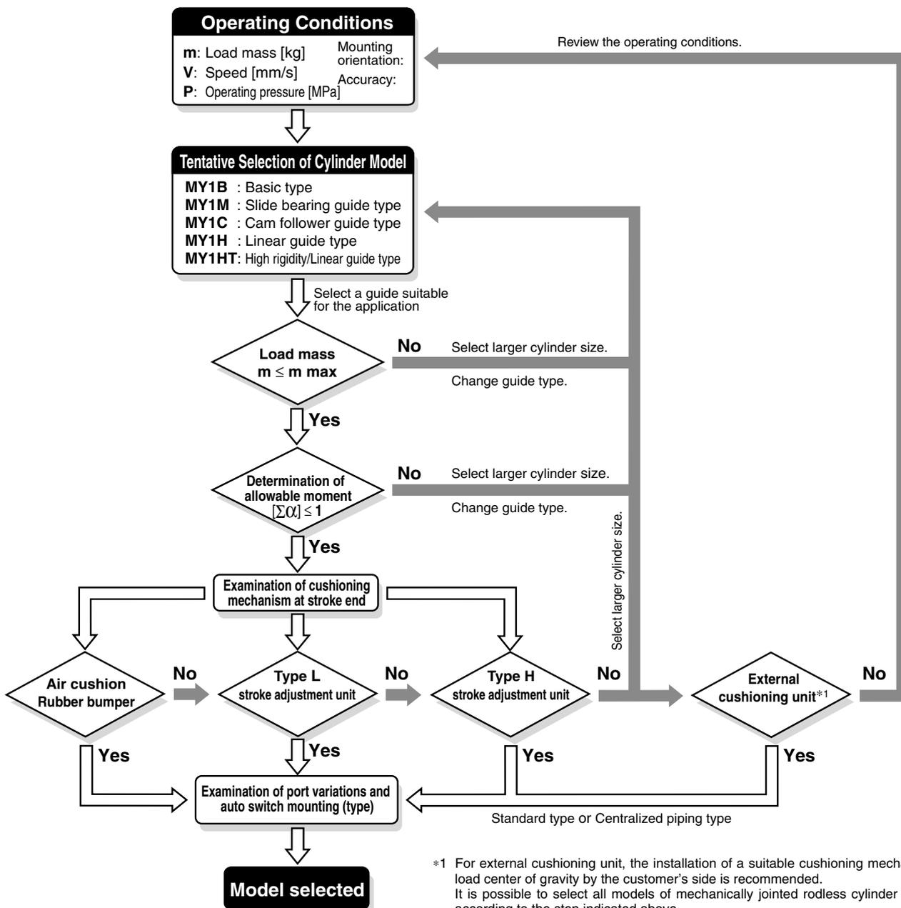
\*1 For external cushioning unit, the installation of a suitable cushioning mechanism near the load center of gravity by the customer's side is recommended. It is possible to select all models of mechanically jointed rodless cylinder (MY1□ series) according to the step indicated above. Refer to the separate operation manual for further details. If you have any questions, please contact SMC.
