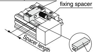
Place the protruding section on the stroke adjustment unit side.
