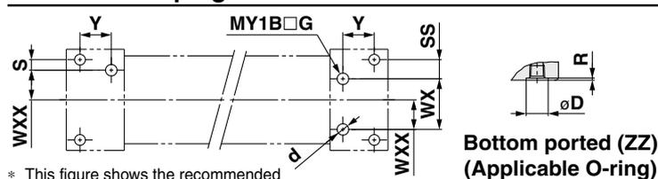
\* This figure shows the recommended machining dimensions of the mounting surface when viewed from the cylinder side.
