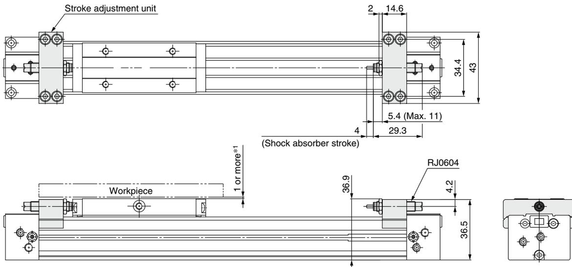
\*1 The clearance between the stroke adjustment unit height dimension (36.9 mm) and the slide table top height (37 mm) is very small, so there is a possibility of interference. For this reason, when mounting a workpiece that exceeds the overall length of the slide table, secure a clearance of 1 mm or more on the workpiece side.
