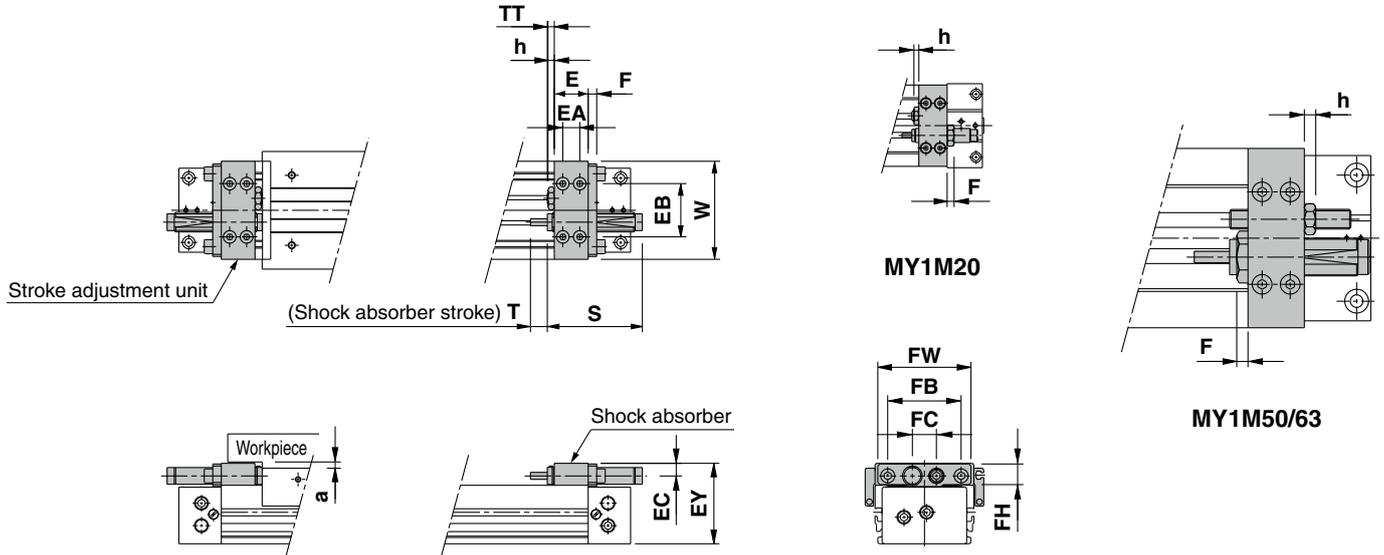
\* Since the EY dimension of H unit is longer than the table top height (H dimension), when mounting a workpiece that exceeds the overall length (L dimension) of the slide table, allow a clearance of dimension "a" or longer on the workpiece side.
