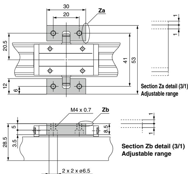
\* Floating brackets consist of a set of right and left brackets.
