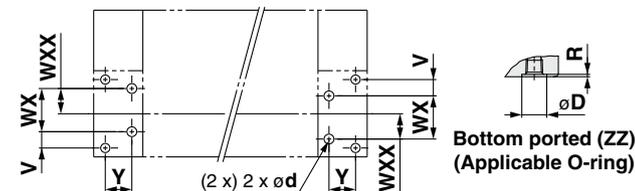
\* This figure shows the recommended machining dimensions of the mounting surface when viewed from the cylinder side.
