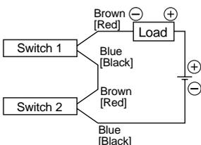
When two switches are connected in series, a load may malfunction because the load voltage will decline when in the ON state. The indicator lights will light up if both of the switches are in the ON state.
