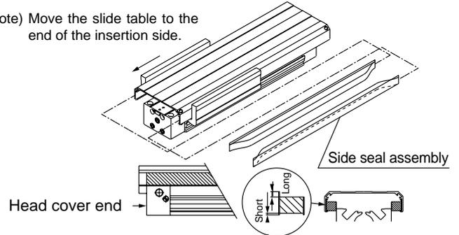
Note) Slide the side seal all the way to the end of the head cover.
