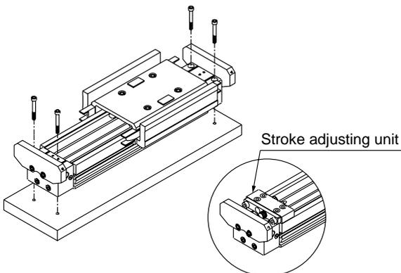
Note) The adjustment of the stroke adjusting unit (optional) should also be done at this time.
