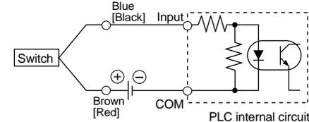
The connection method will vary depending on the applicable PLC input specifications.
