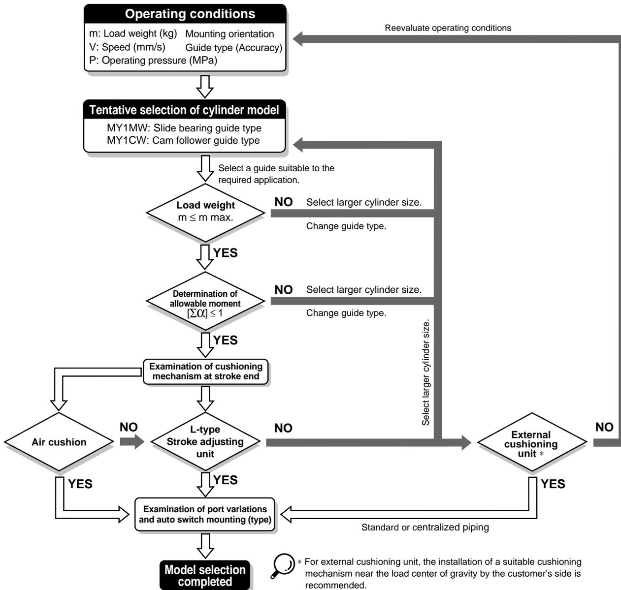
\* For external cushioning unit, the installation of a suitable cushioning mechanism near the load center of gravity by the customer's side is recommended.
