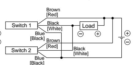
The indicator lights will light up when both switches are turned ON.
