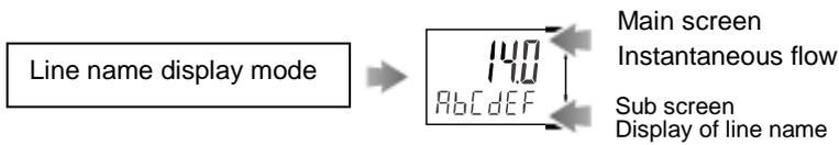
The name of the piping line where the product is installed can be displayed.
