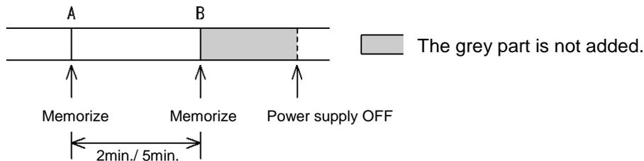
When the power supply is turned on again, the accumulated flow count will start from the last value recorded at B
