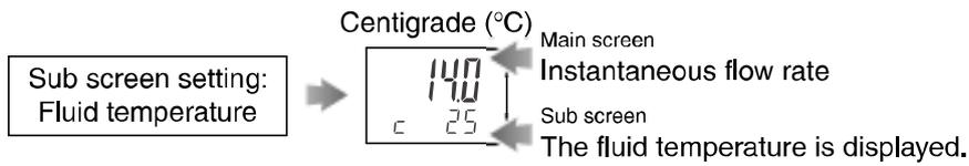
If a fluid temperature sensor is attached, the fluid temperature can be displayed as well.
