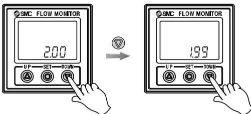
(3) Press the
