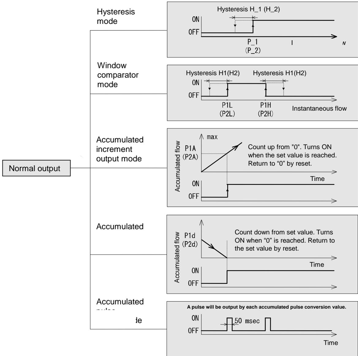
\*: If hysteresis or window comparator mode are selected during unstable flow conditions (due to fluid pulsation, for example), unstable output operation can result.
