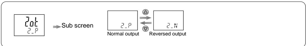
Press the or button to select reversed output mode.
