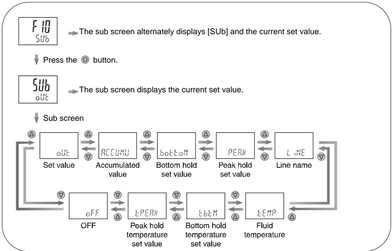
Press the or button to select the desired display.
