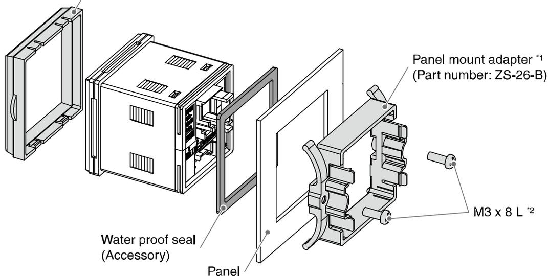
\*1: The panel mount adapter can be rotated through 90 degrees for mounting.
