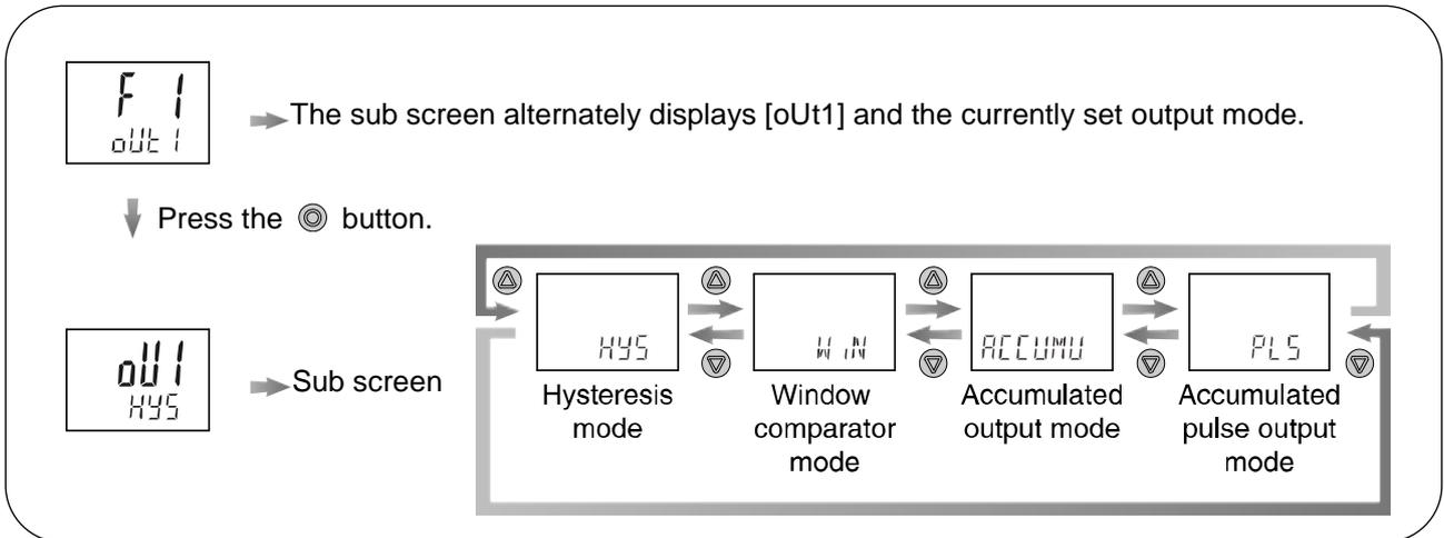
Press the or button to select the desired output mode.
