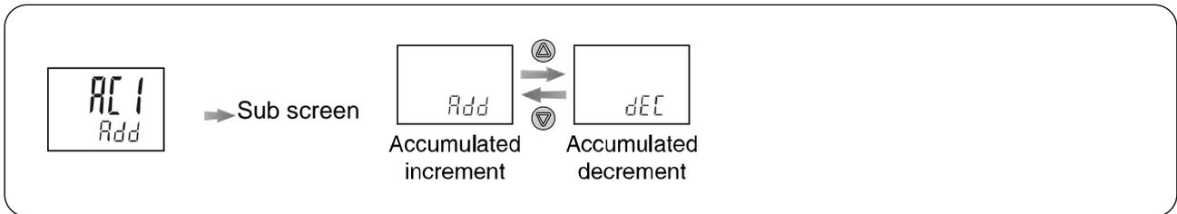
Press the or button to select the desired output mode (Add/dEC).
