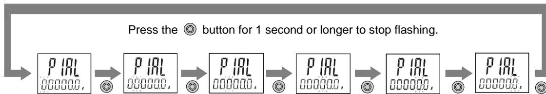
After the input of the lower 6 digits is completed, press the
