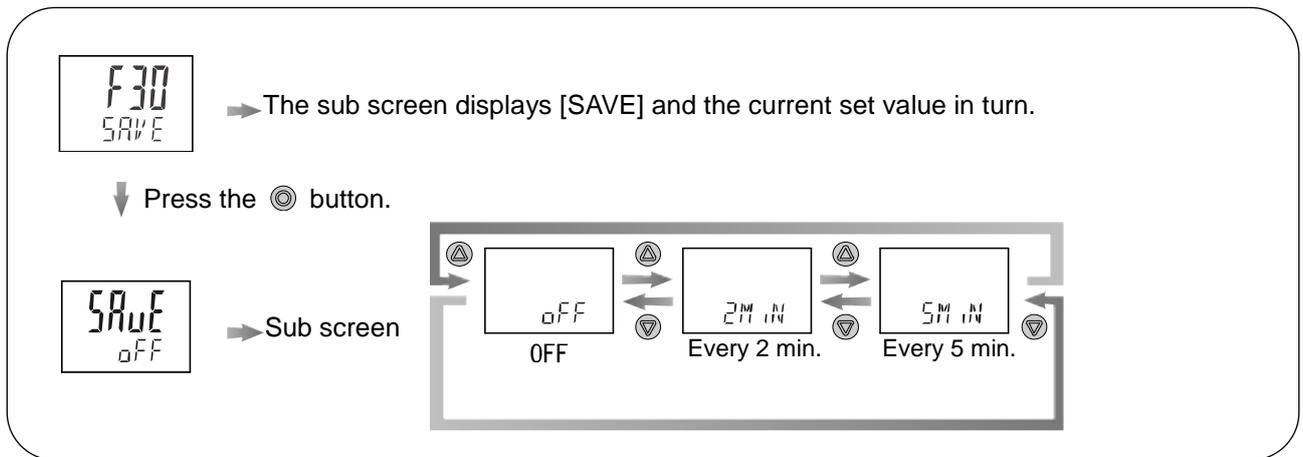
Press the or button to select the accumulate flow value hold.
