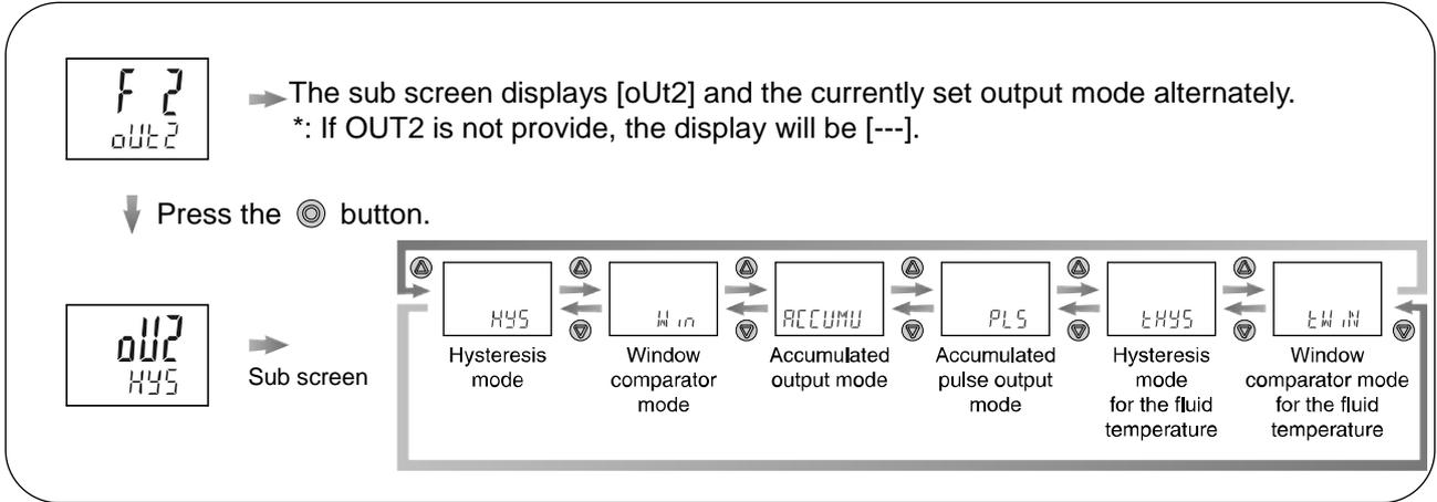
Press the or button to select the desired output mode.
