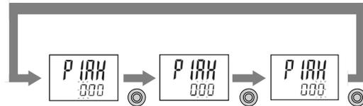
The sub screen displays the set value. The left most digit of the set value will start flashing.
