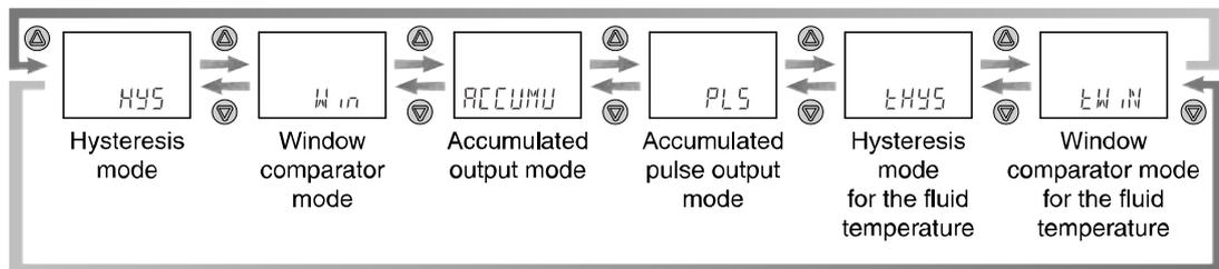
Press the or button to select the output mode.
