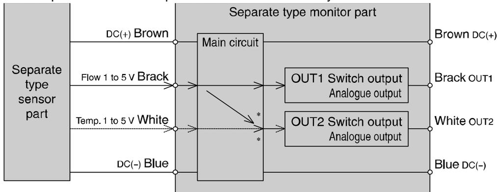
\*: The output at OUT2 can be selected between temperature and flow by setting.
