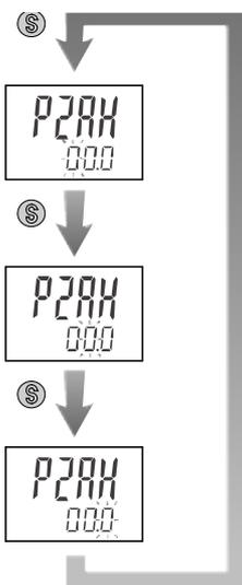
When the **S** button is pressed for 1 second or longer, the flashing will stop.
