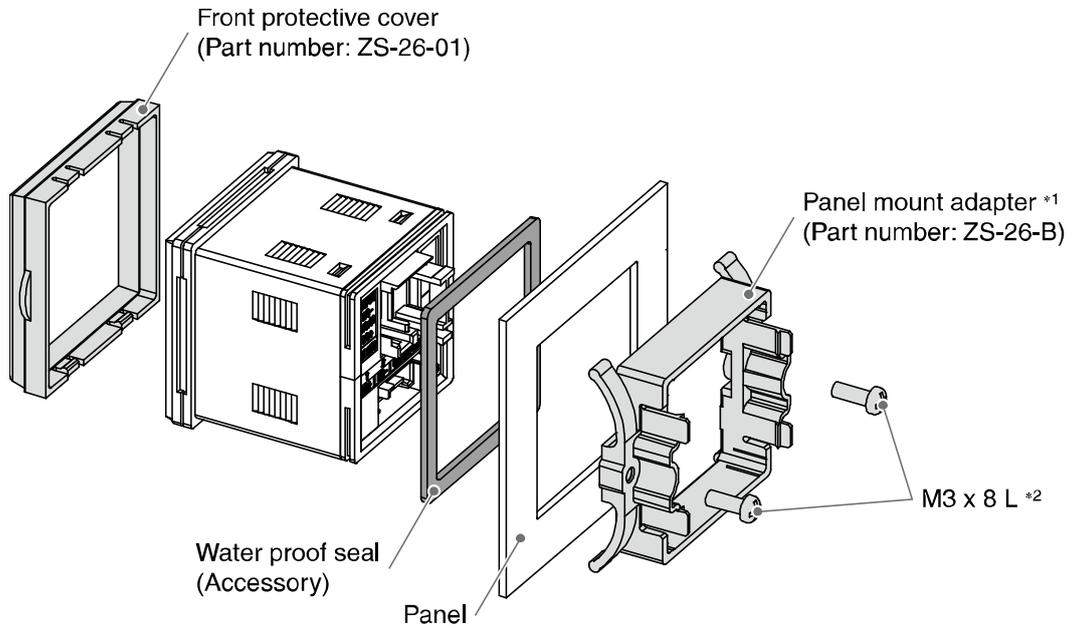
\*1: The panel mount adapter can be rotated through 90 degrees for mounting.
