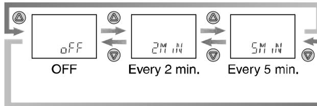
Press the or button to select the setting for storing accumulated flow.
