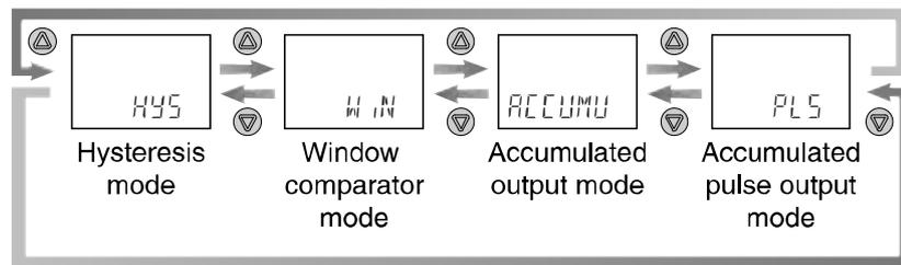
Press the or button to select the output mode.
