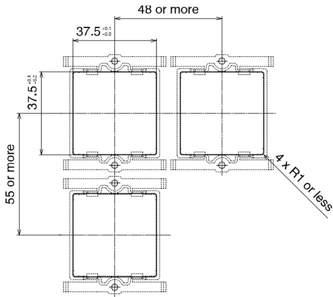
\*: The thickness of the panel is 0.5 to 8 mm (with a waterproof seal: 0.5 to 6 mm)
