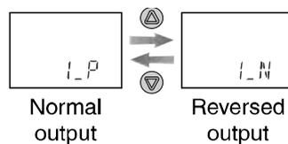
Press the or button to select the switch operation.
