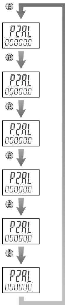
When the **S** button is pressed for 1 second or longer, the flashing will stop.
