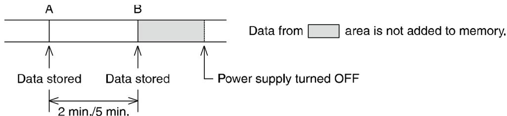
When the power supply is turned on again, the accumulated flow count will start from the value recorded at B.
