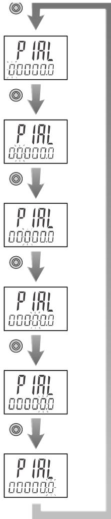
The sub screen displays the value, and the leftmost digit of the set value will start flashing.
