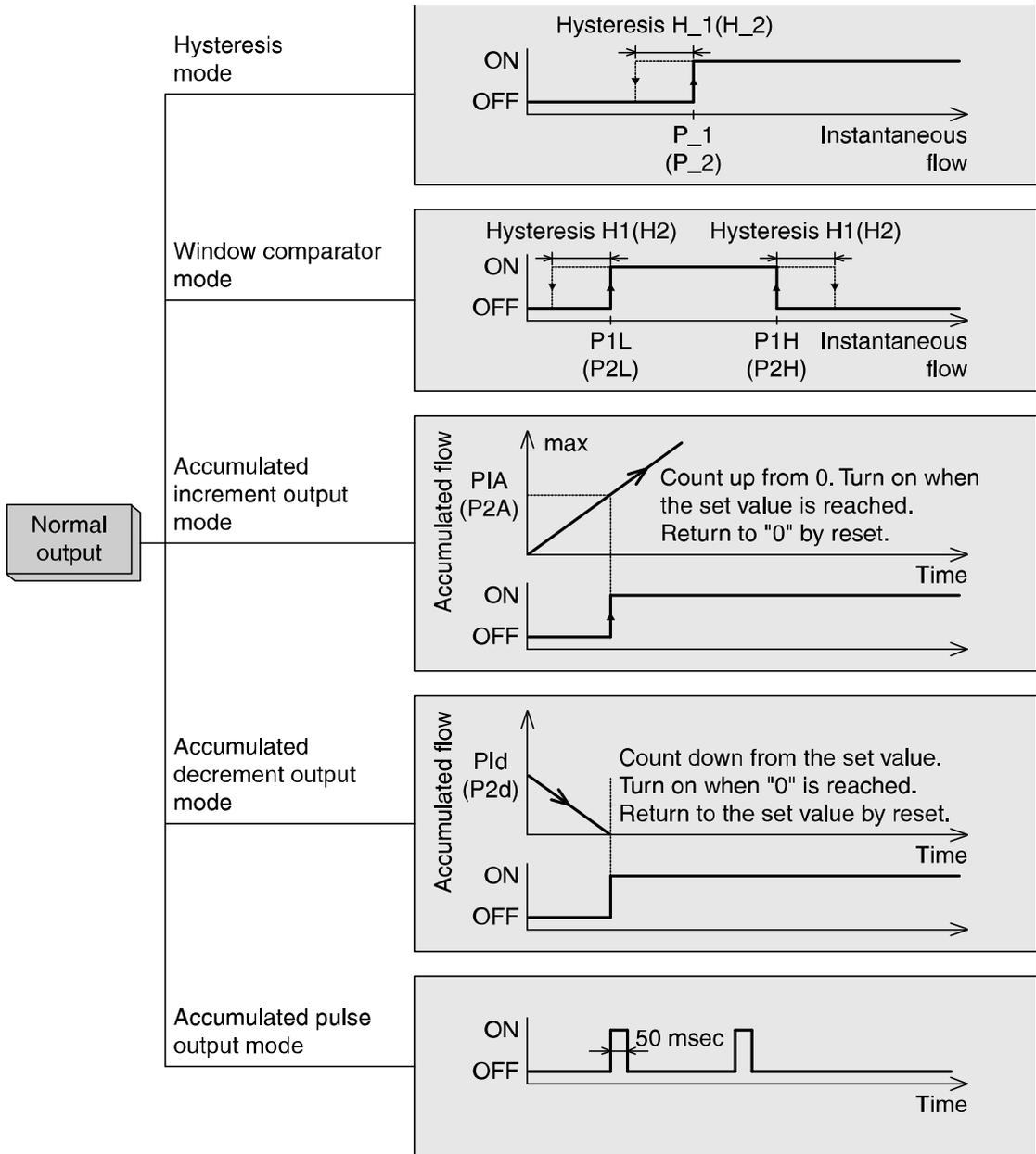
\*: If hysteresis or window comparator mode is selected and there is an unstable flow condition (due to fluid pulsation, for example), unstable output operation can result.
