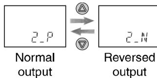
Press the or button to select switch operation.
