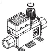
The flow adjustment valve is not designed for applications that require daily and repetitive adjustment. If the valve is adjusted frequently, fluid may leak due to wear of the internal seal.
