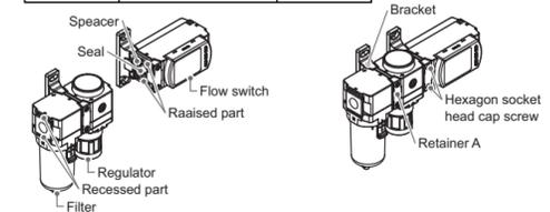
The following options are required for coupling with modular F, R, and L combinations. They are separately prepared by the user.
