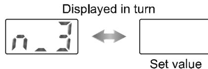
\*: When Non-Reverse output is selected as the switch operation, [P\_3] is displayed.
