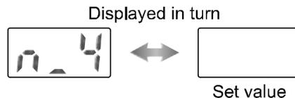
\*: When Non-Reverse output is selected as the switch operation, [P\_4] is displayed.
