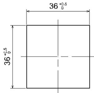
\*: Suitable for panel thickness of 1 to 3.2 mm.
