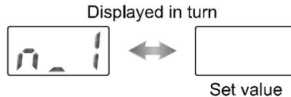
\*: When Non-Reverse output is selected as the switch operation, [P\_1] is displayed.
