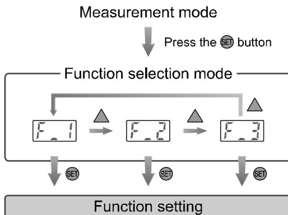
\*: When OUT1 or OUT2 is assigned to be instantaneous output mode during initialize mode, [F\_1] and [F\_2] are displayed.
