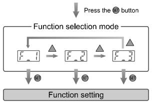
\*: When OUT1 or OUT2 is assigned to be instantaneous output mode during initialize mode, [F\_1] and [F\_2] are displayed. When OUT1 or OUT2 is assigned to be accumulated output mode, [F\_3] is displayed.
