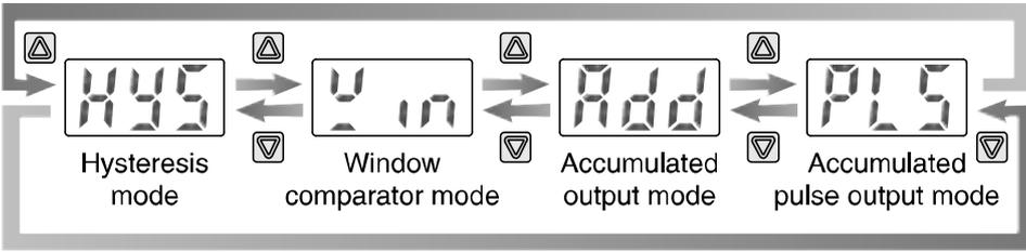
Hysteresis mode      Window comparator mode      Accumulated output mode      Accumulated pulse output mode
