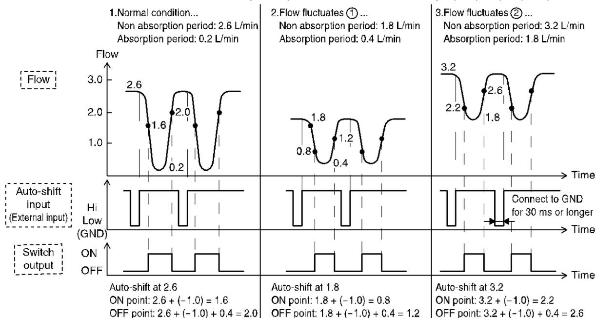
The table below shows an example of the flow displayed when auto-shift zero is selected. Here, a typical condition is used as an example
