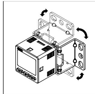
\*Bracket can be mounted on 4 sides.
