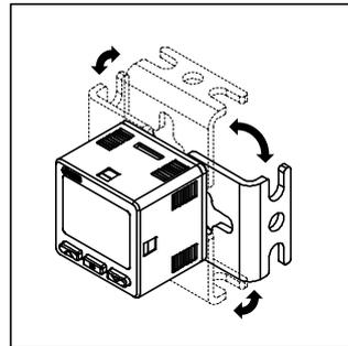
\*Bracket can be mounted on 4 sides.
