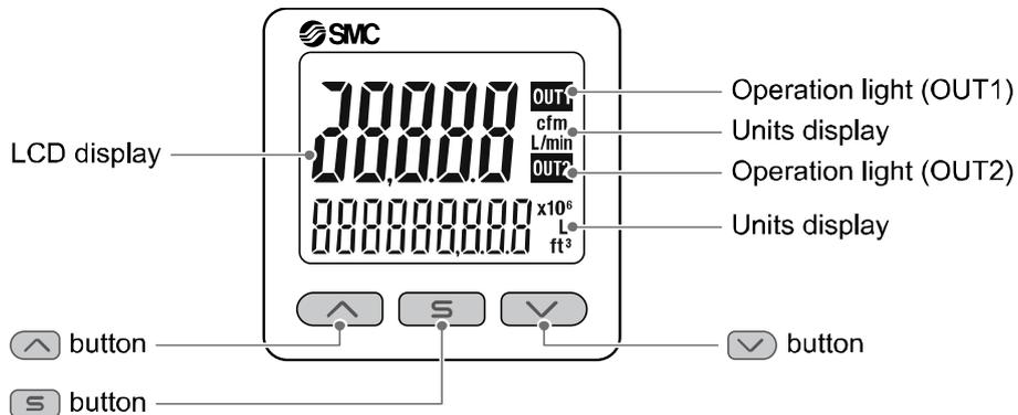
**Operation light:** Displays the switch operating condition.
