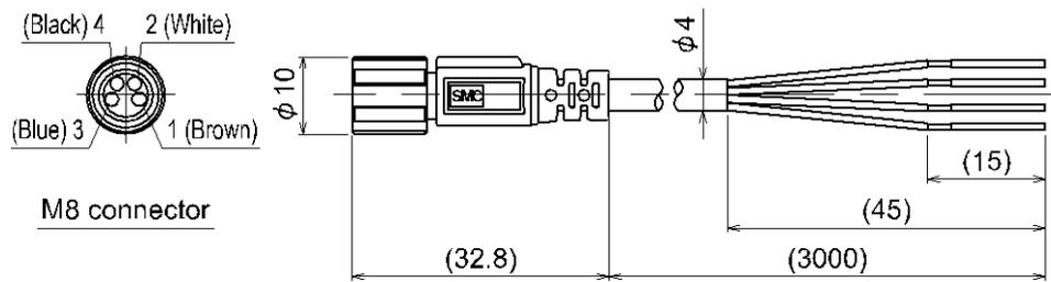
**Dimensions of lead wire with M12-M8 connector (ZS-40-M12M8-A)**
