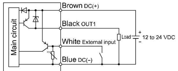
Example of wiring for accumulated pulse output
