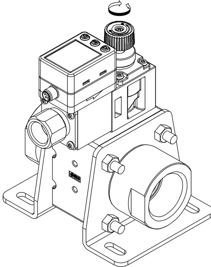
The flow adjustment valve is not designed for applications that require daily and repetitive adjustment. If the valve is adjusted frequently, fluid may leak due to wear of the internal seal.
