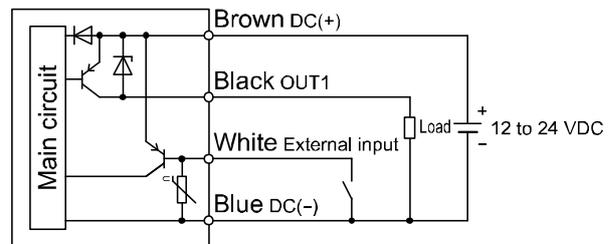
Example of wiring for accumulated pulse output
