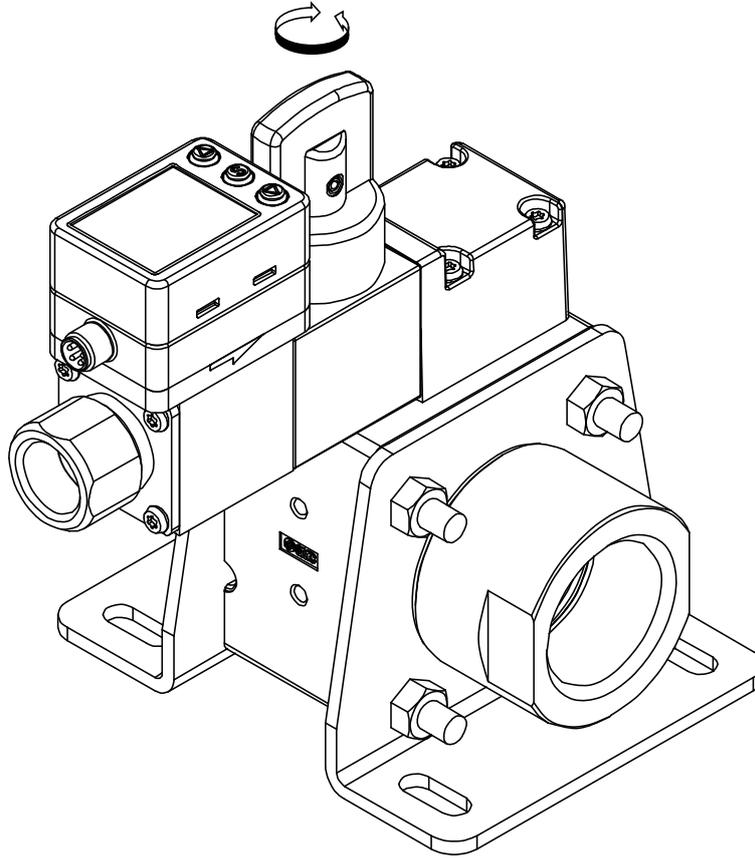
When closing and opening are repeated frequently, water leakage may occur due to wear of the internal seals.
