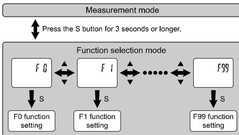
Press the S button for 2 seconds or longer to return to measurement mode.
