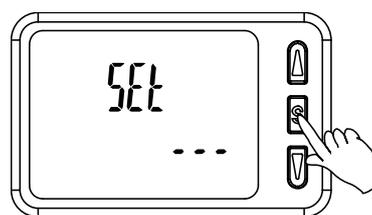
\*: When [F 1] and [F 2] are set to accumulated pulse output, error output or output OFF [---] will be displayed in the sub screen when [SEt] is displayed. It is not possible to move to the Simple setting mode.
