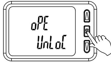
(2) Select the key locking/un-locking using the ▲ or ▼ button, and press the S button to set.
