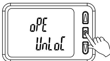
Press the ▲ or ▼ buttons simultaneously for 5 seconds or longer.
