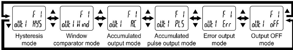
Press the S button to set. ↓ Move on to select normal output/reversed output.
