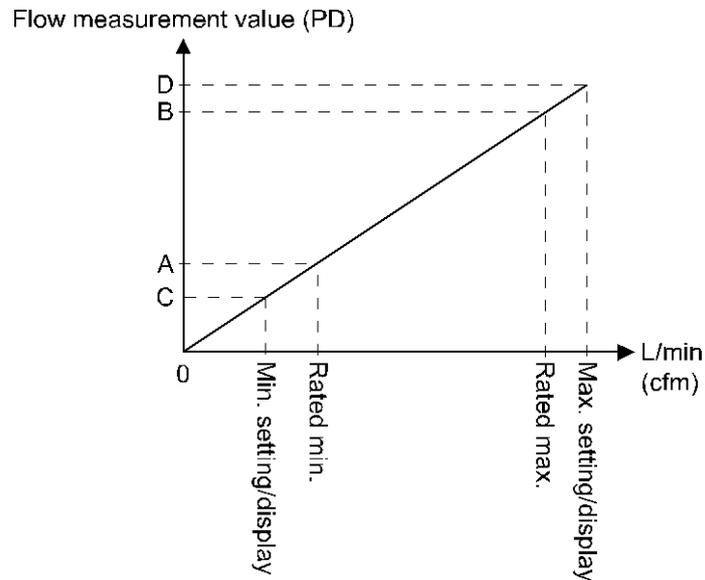
○ Conversion formula of the process data and flow measurement value
