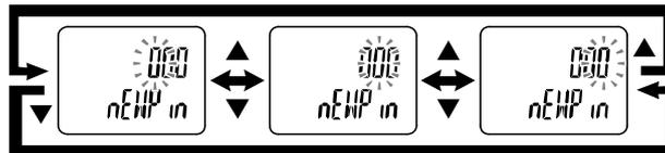
After entry, the changed security code will flash by pressing the S button for 1 second or longer.
