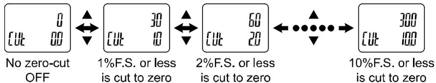
\*: The display above is an example of when [L] is selected for the PF3A703H (3000 L/min type) with the unit switching function.
