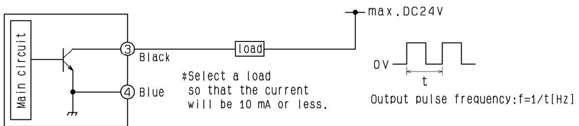
Wiring example of the output signal
