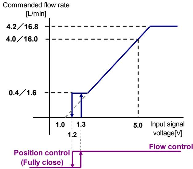
Graph 1: Input signal – Flow characteristics
