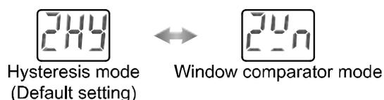
Press the SET button to set the operation mode, and the output style of OUT2 option will appear.
