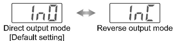
2) The operating mode and the output style for OUT2 is set. (only CH1)
