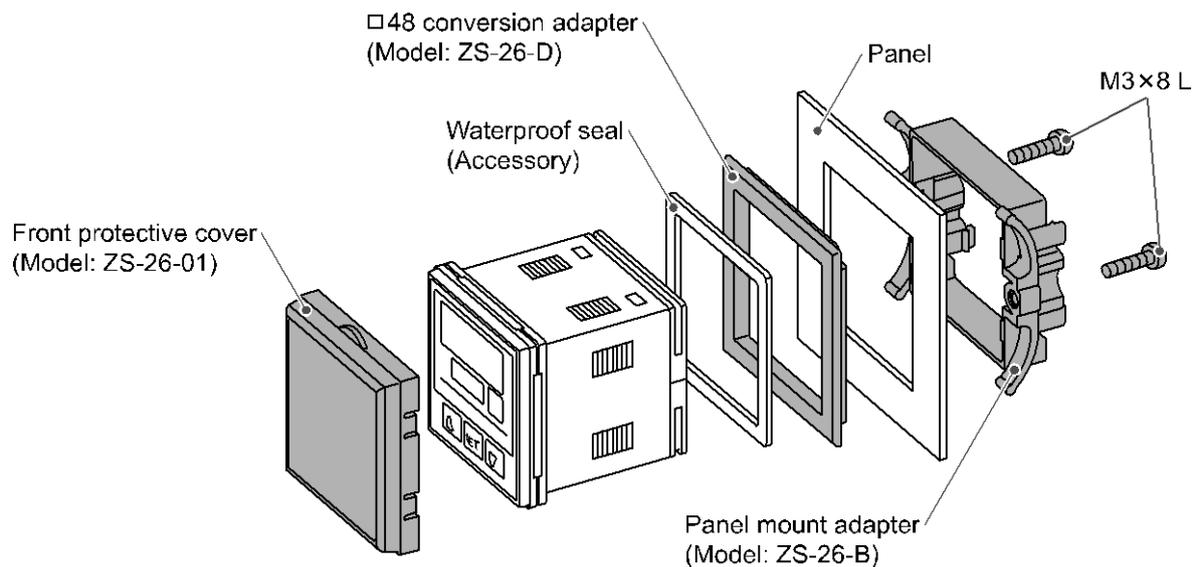
\*: The panel mount adapter can be rotated by 90 degrees for mounting.
