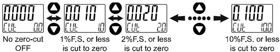
\*: The display above is an example of when [MPa] is selected for the ISE70 (1 MPa range) with the unit switching function.
