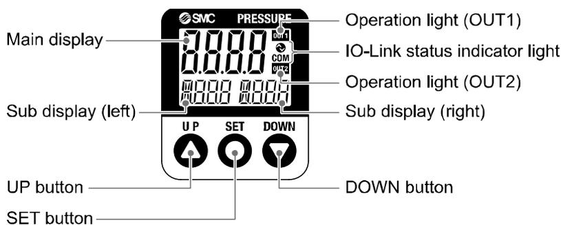
Operation light: Displays the switch operating condition.
