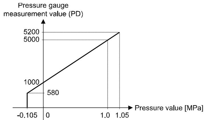
Relationship between the pressure gauge measurement value (PD) and pressure value (e.g.: ISE70 unit MPa)
