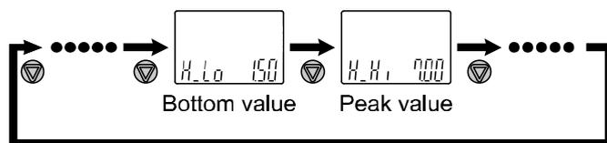
When the SET and DOWN buttons are pressed for 1 second or longer simultaneously while the peak/bottom values are displayed, the sub display (right) displays [- - -] and the maximum (minimum) pressure value are cleared.
