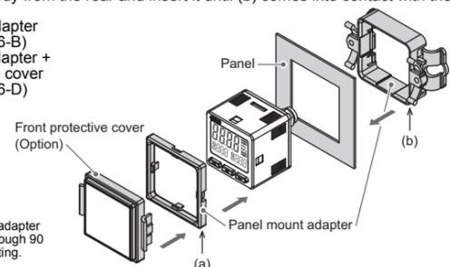
\*: The panel mount adapter can be rotated through 90 degrees for mounting.
