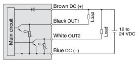
Max. applied voltage: 28 V, Max. load current: 80 mA, Internal voltage drop: 1 V or less
