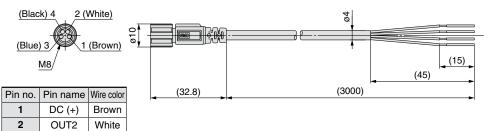
Blue Note) 4-wire type lead wire and M8 connector used for the PFMC7 series. Note) Refer to the Operation Manual in our website for wiring. Black
