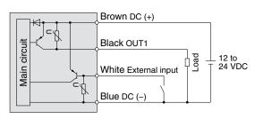
Max. load current: 80 mA, Internal voltage drop: 1.5 V or less External input: input voltage 0.4 V or less (reed or solid state input) for 30 msec. or longer
