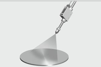
When the product is used for blowing, use caution to prevent the workpiece from being damaged by air entrained from the surrounding area.
