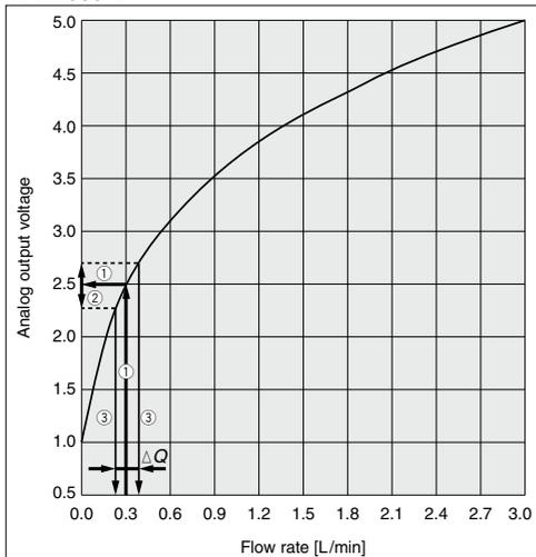
When the flow rate display function for the PFMV3 series is selected, calculate the repeatability from the analog output characteristics graph (page 294).
