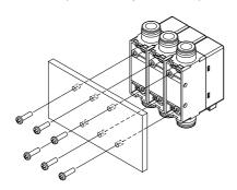
4. When fixing the switch with screws using mounting holes, use a tightening torque of 0.3 N⋅m or less. If necessary, tighten the product to prevent it from loosening.
