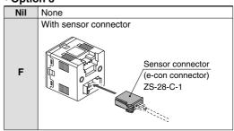
Note) Connector is not connected, but shipped together.
