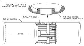
Single melt 316L SS was the semiconductor industry standard for material until the early 90's. Two primary factors were the driving forces behind the quantum shift to secondary remelt (VAR) material. One factor was the desire for finer and finer surface finishes with enhanced surface chemistry. VAR material is more homogeneous than single melt, which enables mirror like surface finishes unattainable with single melt. Lower impurities coupled with finer
