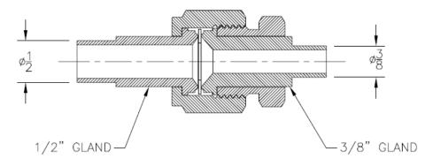
AP Tech's standard for 1/4 inch face seal fittings are the high flow type. The 3/8 inch size fittings are used on products when a 1/2 inch size fitting is desired and the smaller bore size of the 3/8 compared to a 1/2 inch fitting does not restrict flow through the device.
