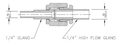
The differences between a 3/8 inch and 1/2 inch face seal fitting are basically the same as the 1/4 inch example above. The nuts, gasket and sealing bead geometries are the same. The physical differences are the through bore diameter and the weld size, with each welding to the same size tubing as the fitting size designation. The two fittings mate with each other.
