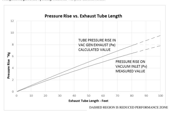
For example, a vacuum generator is installed to evacuate process gas. The initial rough installation is done with no exhaust tube, exhausting directly to atmosphere (Pe=0"Hg). Vacuum inlet pressure (Pi) is measured to be -26"Hg with no inlet flow. To safely exhaust process gases to a scrubber, 10 feet of straight 3/8" exhaust tube is added. Exhaust pressure rises to 1"Hg (0.53 psig) at the generator and Pi rises by a similar amount delivering nearly -25"Hg with no inlet flow.
