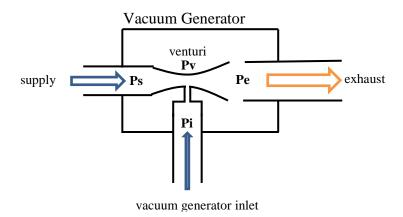
a short narrow passage called a venturi. Ps must be sufficient to ensure choked flow in the venturi throat. Choked flow is present for gases with k=1.4 when the absolute pressure ratio Pe/Ps < 0.528 (critical pressure ratio). Choked flow maximizes gas velocity and results in the lowest achievable Pi. If not maintained, Pi becomes unstable with loss of vacuum. When accelerated, much of the gas potential energy (pressure) is converted to velocity. Due to
