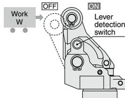
When the lever stands erect (when the energy is absorbed), the switch turns on a signal that determines the pallet has reached the stop position. (For details of lever detection switch, refer to page 595.)
