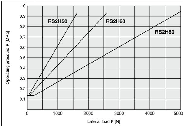
Even after the impact of the carried object is absorbed, lateral load acts on the stopper cylinder due to the friction generated between the conveyor and the carried object.
