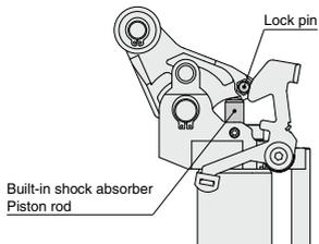
Similarly, be careful not to remove the grease from the piston rod end of the built-in shock absorber. Check the grease application state periodically.
