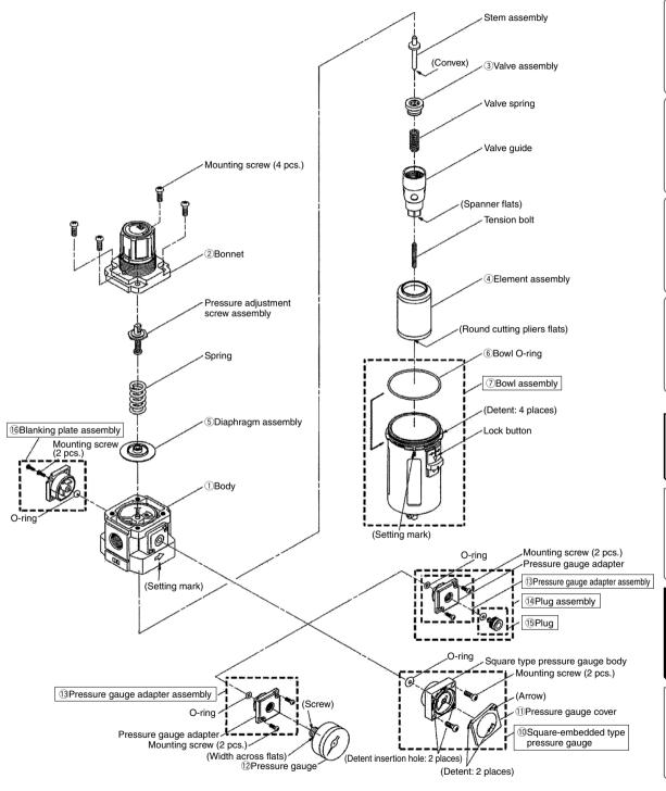
Note) It is possible to mount a  $\mathbin{\textcircled{\scriptsize 10}}$  square-embedded type pressure gauge, a  $\mathbin{\textcircled{\scriptsize 3}}$  pressure gauge adapter assembly, or a 4 plug assembly instead of a 6 blanking plate assembly.
