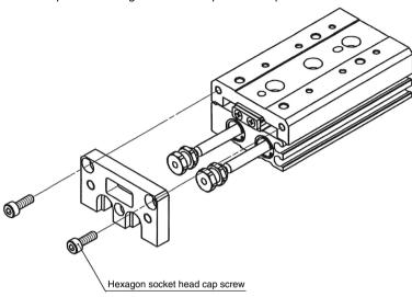
Apply Henkel Japan Loctite No.262 or an equivalent adhesive.
