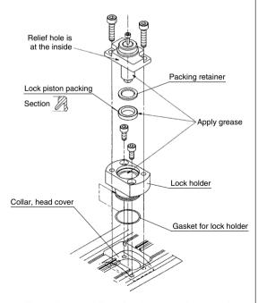
Fig. 12 Reassembling of end lock part (Ø80, Ø100)
