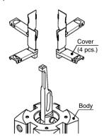
3) After cleaning the adhesive from the hexagon head bolts (4 pcs.) and the body with alcohol etc., apply the tightening adhesive to the screw holes of the body (SMC recommended adhesive: Loctite Corp. 262 [Red]) in order not to loose. Spread lithium system grease on the pin hole part of pin A and the guide tube.
