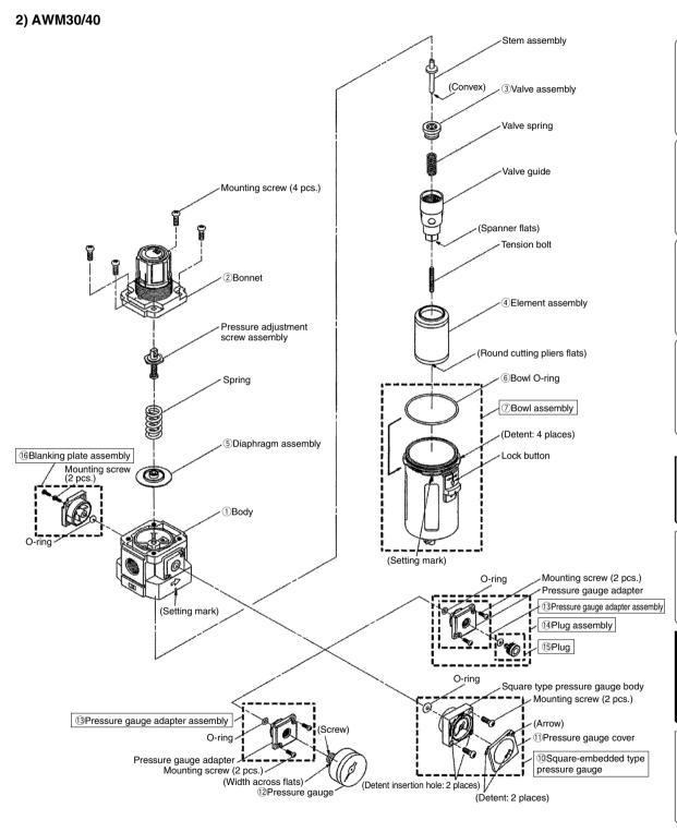
Note) It is possible to mount a (1) square-embedded type pressure gauge, a (1) pressure gauge adapter assembly, or a (1) plug assembly instead of a (1) blanking plate assembly.
