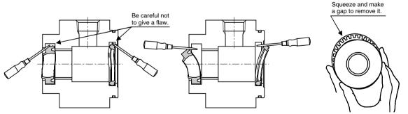
Fig. 1 Removal of rod seal and cushion seal
