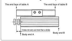
Make sure that table end A does not exceed the body end A at the full stroke after removing the end plate. Make sure that table end B does not exceed the body end B at the full stroke after removing the end plate. (The steel balls in the guide will fall out.)
