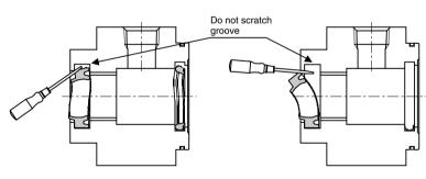
Fig. 1 Removal of rod seal
