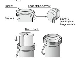
\* Set the handle avoiding attaching it to the notch (guide slit) of the case and INLET.
