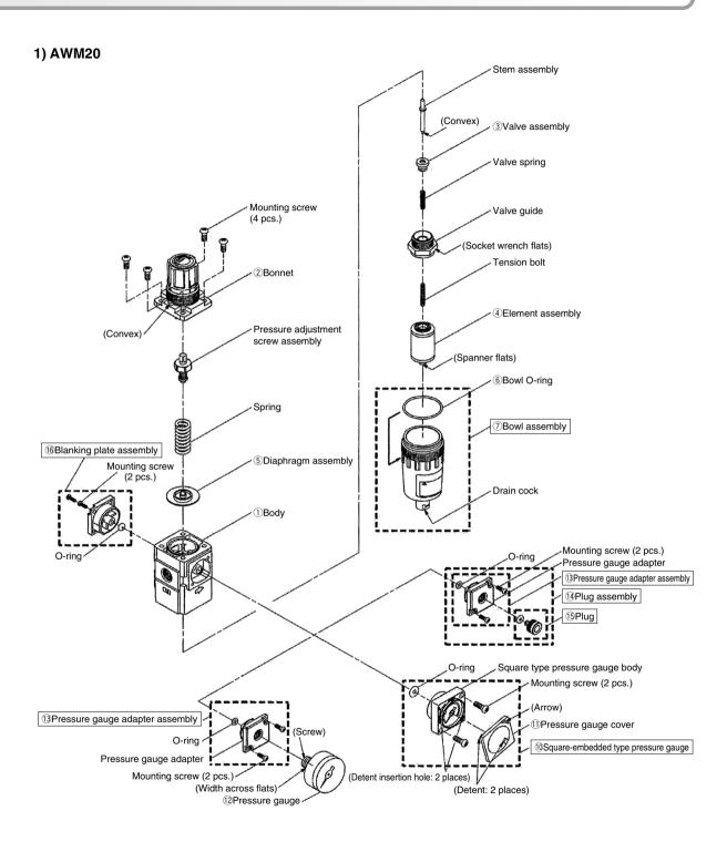
Note) It is possible to mount a <sup>®</sup> square-embedded type pressure gauge, a <sup>®</sup> pressure gauge adapter assembly, or a <sup>®</sup> plug assembly instead of a <sup>®</sup> blanking plate assembly.
