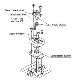
Fig. 14 End lock reassembled (Ø50, Ø63)
