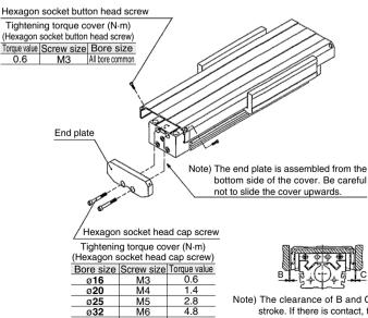
Note) The clearance of B and C part has to be checked at the full stroke. If there is contact, the clearance should be adjusted by loosening the hexagon head cap screw and retightening it.
