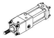
b. Remove the tie rods, head cover and cylinder tube.
