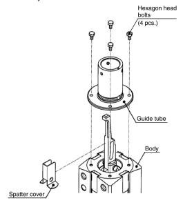
3) Insert a flat blade screwdriver or similar object into the cover groove and open. Then detach the cover (4 pcs.).
