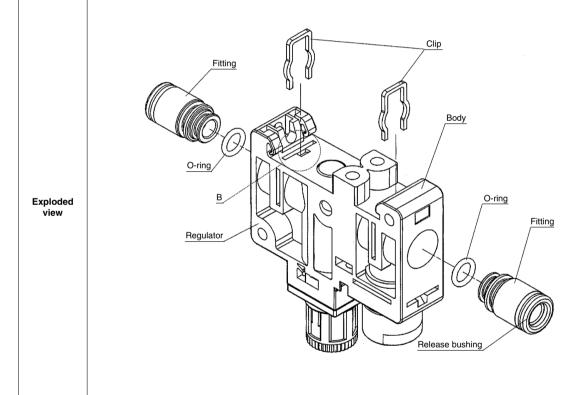
\* If it is hard to remove the fitting, do not remove the release bushing with a strong force. It that case, install the tube and plug, and pull the fitting out together with them.
