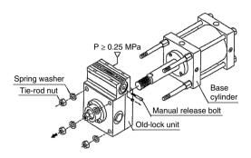
4-4. Remove four holding bolts for the new lock unit brake tube assembly and remove the brake tube assembly.
