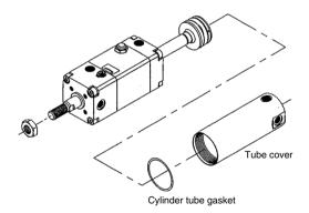
8-3. Apply compressed air of 0.3 MPa or more to the unlocking port, and pull out the piston rod assembly.
