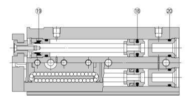
\* The numbers correspond with those in the "Construction" of the MXQR series in the Best Pneumatics catalog.
