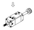
Note) When replacing piston rod assembly with a new lock unit, care should be taken not to cut rod packing B with threads or wrench flats.
