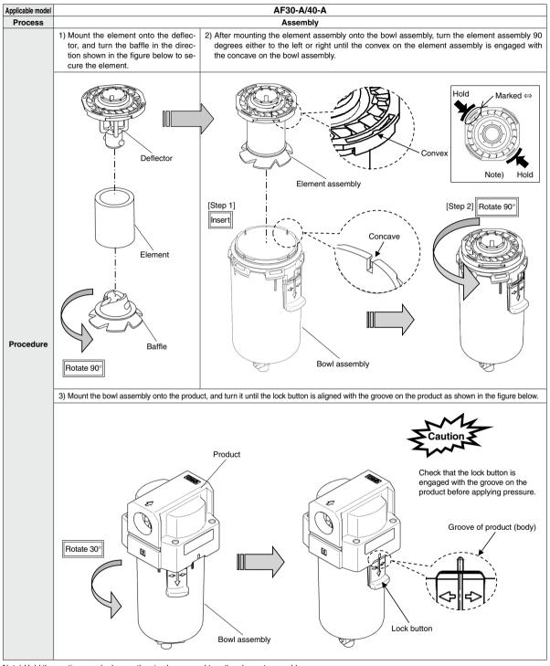
Note) Hold the sections marked  $\Leftrightarrow$  on the circular arc, and turn the element assembly.
