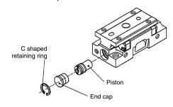
1-4. Apply grease to piston for replacement.
