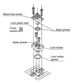
Fig. 13 End lock reassembled (ø32, ø40)
