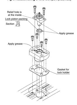
Fig. 11 Reassembling of end lock part (Ø50, Ø63)
