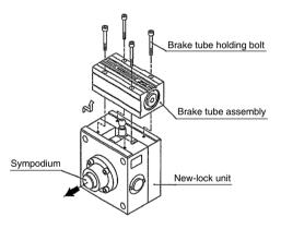
4-5. Pull out the temporary shafts from the lock unit and insert the lock unit to the base cylinder.
