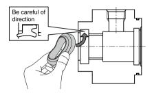
Fig. 4 Installation of rod seal
