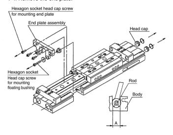
Note) The floating bushing should be mounted/dismounted carefully with a spanner whose width is A to avoid flaws inside the body.
