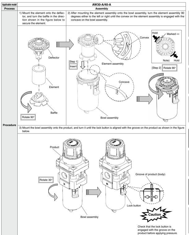
Note) Hold the sections marked ⇔ on the circular arc, and turn the element assembly.
