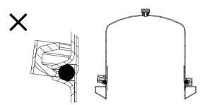
Fig. (b) Incorrect mounting of V-band
