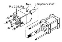
Note) To replace the piston rod assembly with the temporary shaft of a new lock unit, make sure that the compressed air of 0.3 MPa or higher is kept applied to the lock release port.
