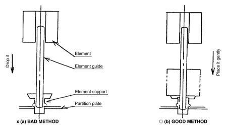
Note) When 2 or 3 elements are put one upon another, it is possible to firstly set elements and joints to the element guide and then mount the element guide assembly on the element support. (Refer to Fig. 1, reversely to the order of removal.)
