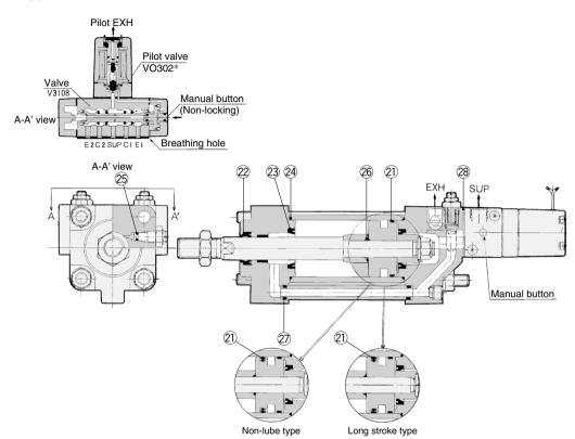
\* The numbers correspond with those in the "Construction" of the CV3 series in the Best Pneumatics catalog.
