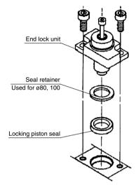
Fig. 1 How to remove the end lock
