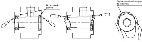
Fig. 1 Removal of rod seal, cushion seal
