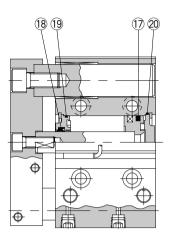
\* The numbers correspond with those in the "Construction" of the MGPS series in the Best Pneumatics catalog.
