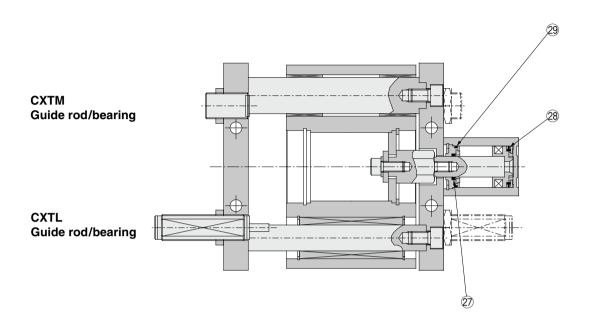
\* The numbers correspond with those in the "Construction" of the CXT series in the Best Pneumatics catalog.
