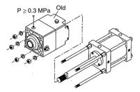
c. Also apply compressed air over 0.3 MPa to new lock unit and replace piston rod of cylinder with temporary shaft.
