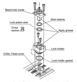
Fig. 15 End lock reassembled ( $\emptyset 80, \emptyset 100$ )
