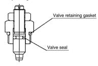
Fig. 4 Positions of valve seal and valve retaining gasket
