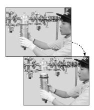
1-6. Clean the inside of the case, gaskets, seals, holders, plugs, etc., with a pure fluid or solvent.
