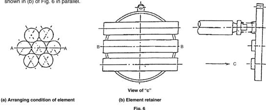
Note 1) When the element retainer is installed, place it correctly in such a way that the element mounting bracket is not moved.
