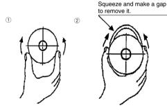
Fig. 2 Removal of piston seal
