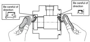
Fig. 4 Mounting of rod seal, cushion seal
