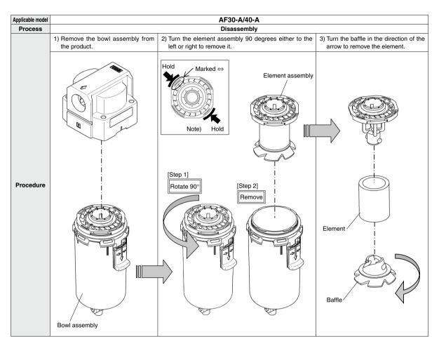
Note) Hold the sections marked  $\Leftrightarrow$  on the circular arc, and turn the element assembly.
