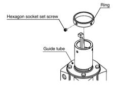
5) Insert the replacement parallel pin in the pin hole of the replacement guide assembly (when equipped with a shim, secure with adhesive on the parallel pin and the guide pin assembly), line up with the pin hole on the guide tube, insert, and tighten with the hexagon socket set screw (3 pcs.: with the adhesive [Green]).
