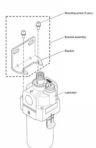
AL20-A to 60-A Bracket Assembly Exploded View 4
