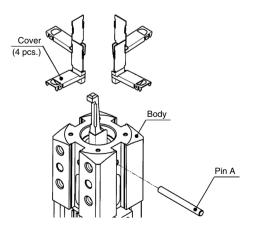
3) Loosen the hexagon socket head cap screw (4 pcs.) the base cylinder, and detach the body from the base cylinder.
