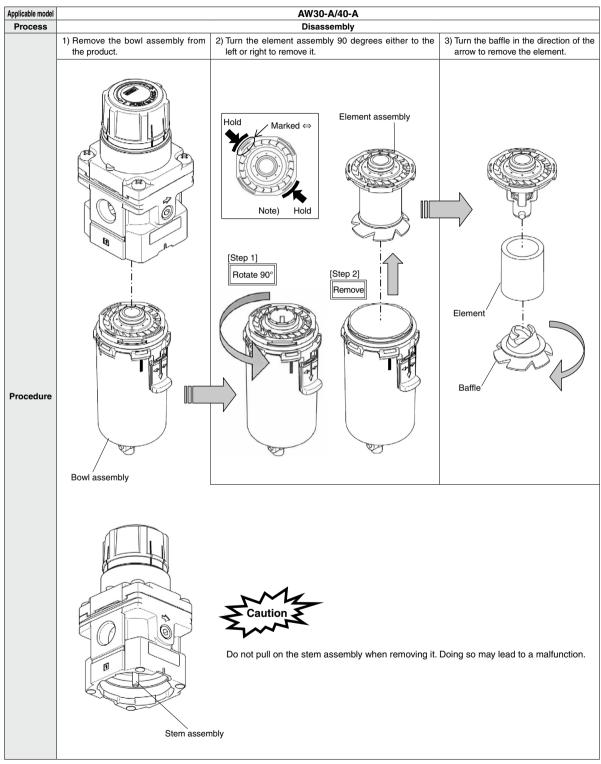
Note) Hold the sections marked  $\Leftrightarrow$  on the circular arc, and turn the element assembly.
