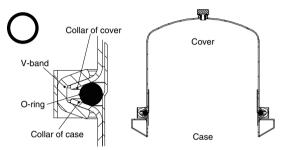
Fig. (a) Correct mounting of V-band
