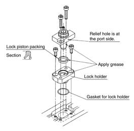
Fig. 9 Reassembling of end lock part (Ø20, Ø25)
