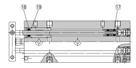
**Dual Rod Cylinder/Basic Type: Slide Bearing**
