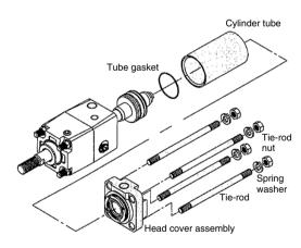
Apply 0.3 MPa or more of compressed air to the unlocking port, and pull out the piston rod assembly.
