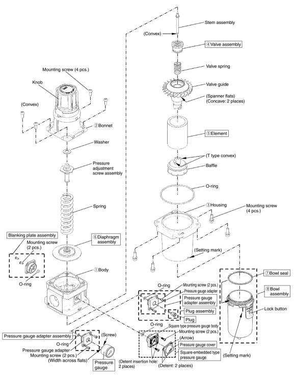
Note) It is possible to mount a square-embedded type pressure gauge, a pressure gauge adapter assembly, or a plug assembly instead of a blanking plate assembly.
