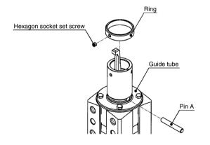
2) Detach the hexagon head bolt (4 pcs.), and detach the guide tube and the spatter cover from the body.
