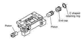
1-7. Apply grease to piston for replacement.
