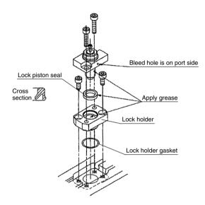
Fig. 12 End lock reassembled (ø20, ø25)
