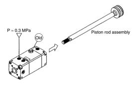
8-4. Similarly apply compressed air of 0.3 MPa or more to the unlocking port of the new lock unit, and replace the temporary axis with the previous piston rod assembly.
