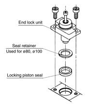
Fig. 1 How to remove end lock
