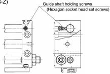
Fig. 2 Set screws for holding the guide shaft
