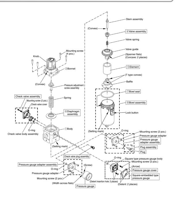
Note) The flow direction can be changed by removing the check valve assembly and replacing it with the square-embedded type pressure gauge, pressure gauge adapter assembly, and plug assembly. At this time, the check valve plug assembly must also be replaced.
