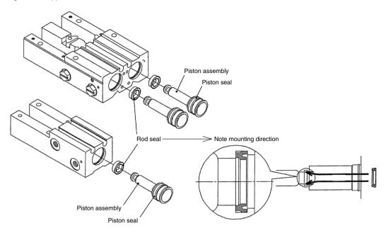
2-5. Apply the specified grease lightly to the sliding interface between the outer periphery and the body of the piston, and assemble them in the reversed order.
