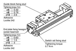
Step between end plate and rail shall comply with table.
