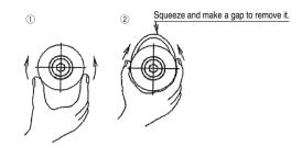
Fig. 2 Removal of piston seal
