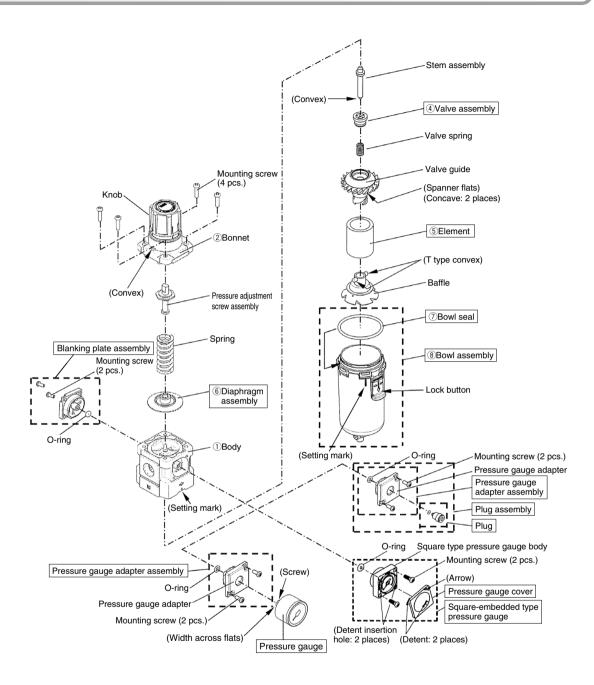
Note) It is possible to mount a square-embedded type pressure gauge, a pressure gauge adapter assembly, or a plug assembly instead of a blanking plate assembly.
