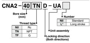
The lock unit for a long-stroke cylinder is only applicable for flange type with bore size ø50 to ø100 and stroke 1001 or more.
