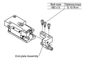
No gap is present at the mating surface between the body assemblies.
