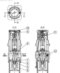
\* The numbers correspond with those in the "Construction" of the AWG series in the Best Pneumatics catalog.
