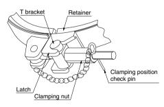
Fig. (c) V-band tightening
