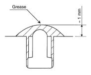
c. Mounting of tube gasket
