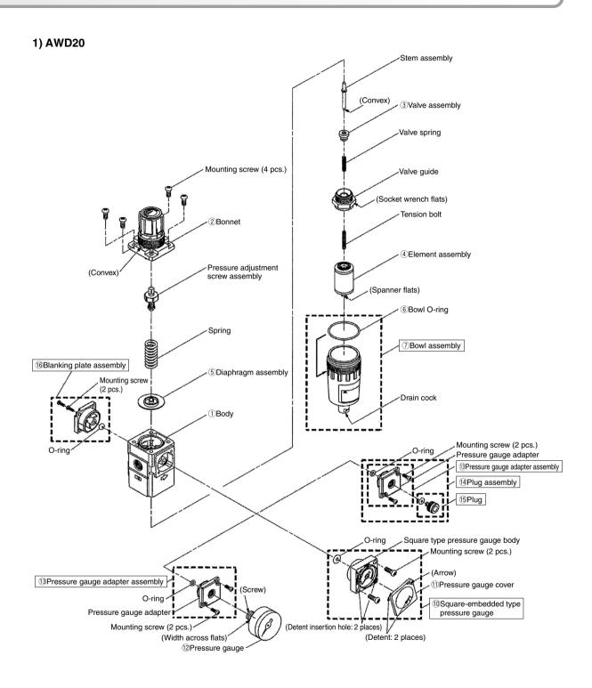
Note) It is possible to mount a 1 square-embedded type pressure gauge, a 3 pressure gauge adapter assembly, or a 4 plug assembly instead of a 6 blanking plate assembly.
