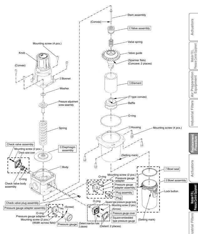
Note) The flow direction can be changed by removing the check valve assembly and replacing it with the square-embedded type pressure gauge, pressure gauge adapter assembly, and plug assembly. At this time, the check valve plug assembly must also be replaced.
