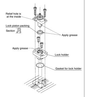
Fig. 10 Reassembling of end lock part (Ø32, Ø40)
