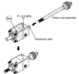
e. Reassemble in reverse order from step b to a.
