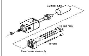
c. Apply 0.3 MPa or more of pressure to the lock release port to pull out the piston rod assembly.
