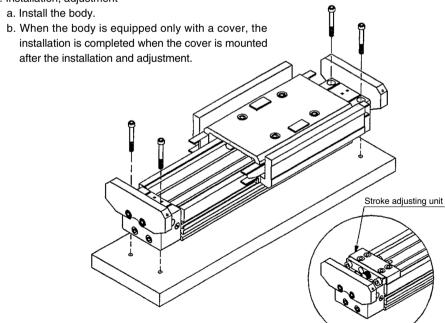
Note) Optional stroke adjustment unit is adjusted here.
