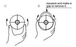
Fig. 3 How to remove piston seal
