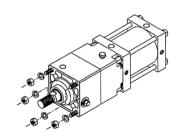
b. Remove lock unit by applying compressed air over 0.3 MPa to lock release port.
