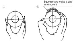
Fig. 3 How to remove piston seal
