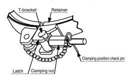
Fig. (c) V-band tightening
