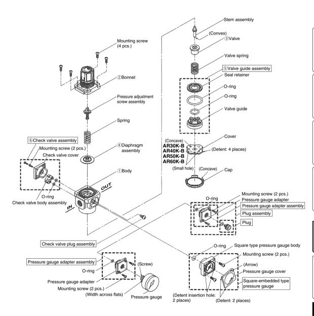
Note) (a) The flow direction can be changed by removing the check valve assembly and replacing it with the square-embedded type pressure gauge, pressure gauge adapter assembly, and plug assembly.
