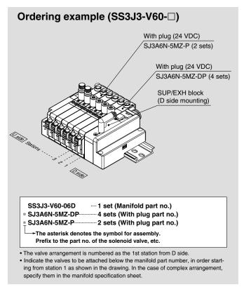
There is no need to enter anything when the SUP/EXH block mounting position "M" is selected. Also, this manifold comes standard with external pilot specifications.
