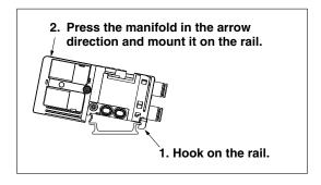
A manifold equipped with a valve or a block assembly can be mounted on the DIN rail. However, a serial connector block assembly cannot be mounted on the DIN rail when it is connected with another block; the serial connector block must be mounted separately.
