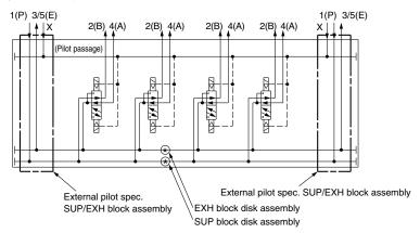
3. Different-pressure spec. using the external pilot (For using the SUP/EXH block assembly for different-pressure internal pilot spec.)
