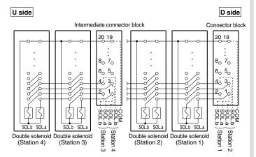
\* Enables control of U side solenoid valves from the position where the intermediate connector block assembly is installed.
