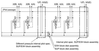
2. Different-pressure spec. using the external pilot (For using the SUP/EXH block assembly for external pilot)
