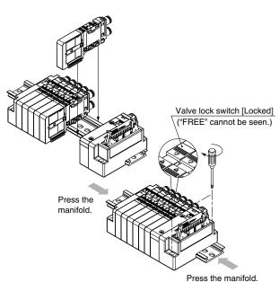
Loosen threads ⓐ, which are fixed onto the DIN rail (two locations on one side).
