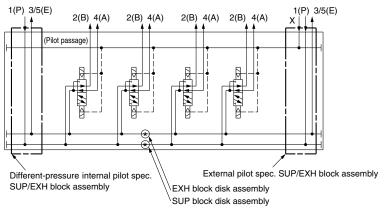
Note 1) When operating under the different-pressure spec., supply the higher pressure to the pilot passage. Note 2) If there is a need to partition the pilot passage, consult SMC.
